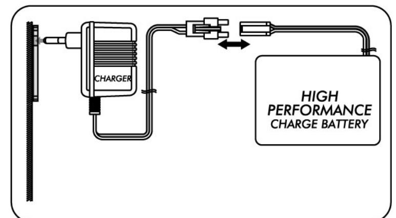
Charge for the 12V, NI-CD 700mAh battery before using. Rechargeable battery:each charge time should be 5 hours. Do not over charge the battery. Approximately play time after each full charge 11 minutes.
