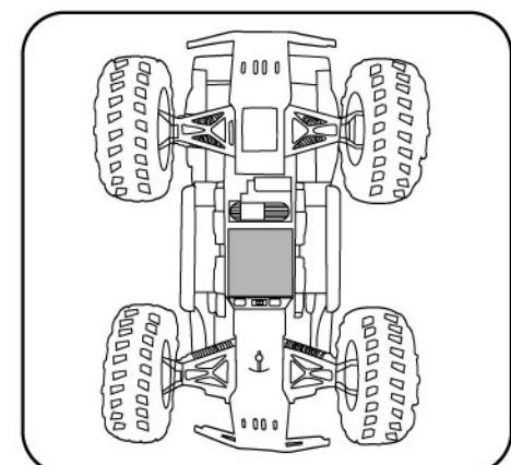
Install 12V 1800mAh battery with polarity (+/-) as shown inside battery compartment and then turn the locking device to lock the battery compartment as shown in picture above.
