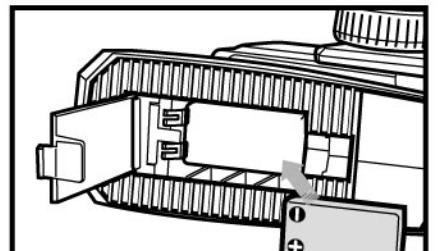
Install one 9V battery with polarity (+/-) as shown inside battery compartment (not included).
