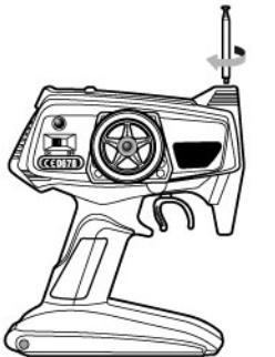
Tighten the antenna into the transmitter.
