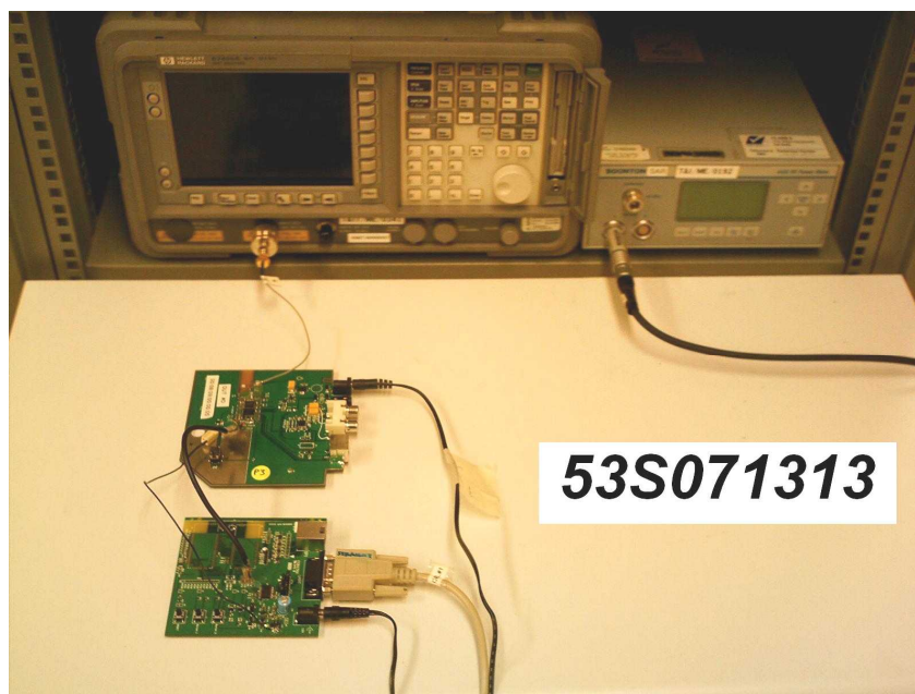
Carrier Frequency Separation Test Setup
