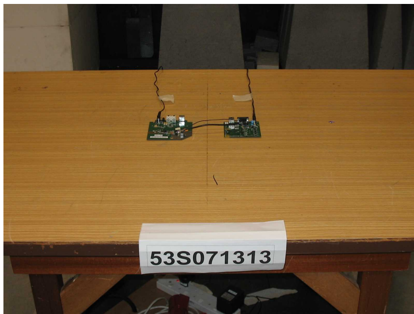
Band Edge Compliance (Radiated) Test Setup
