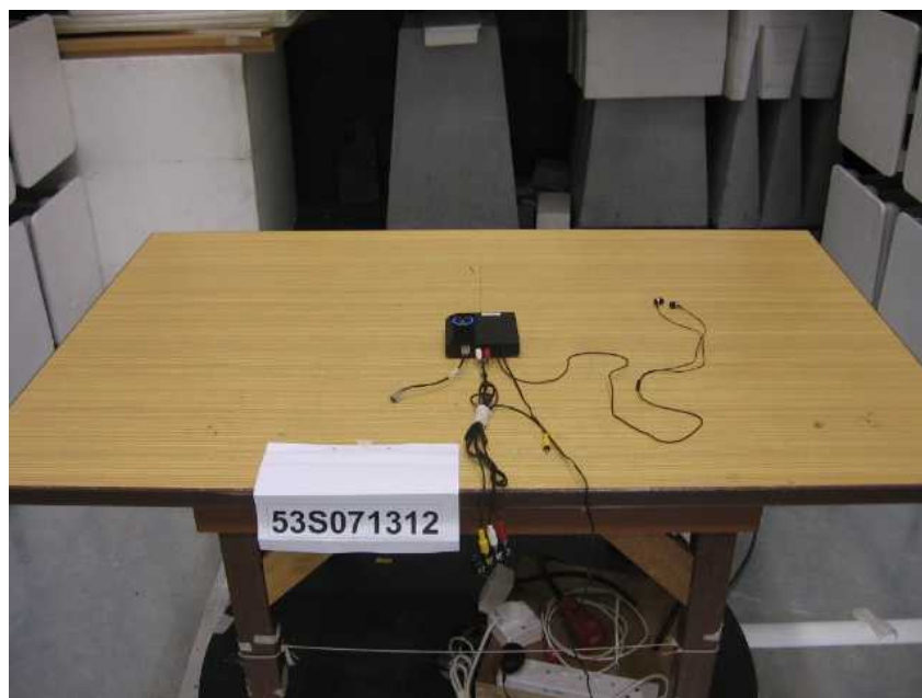
Radiated Emissions Test Setup (Rear View)
