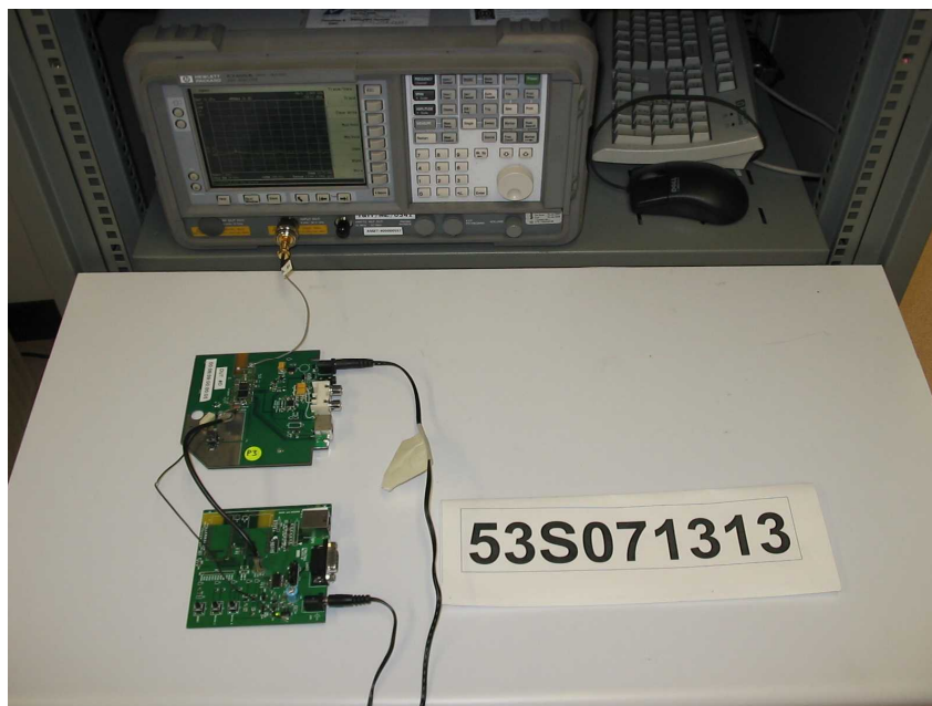
Band Edge Compliance (Conducted) Test Setup
