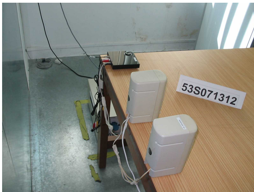
Conducted Emissions Test Setup (Rear View)
