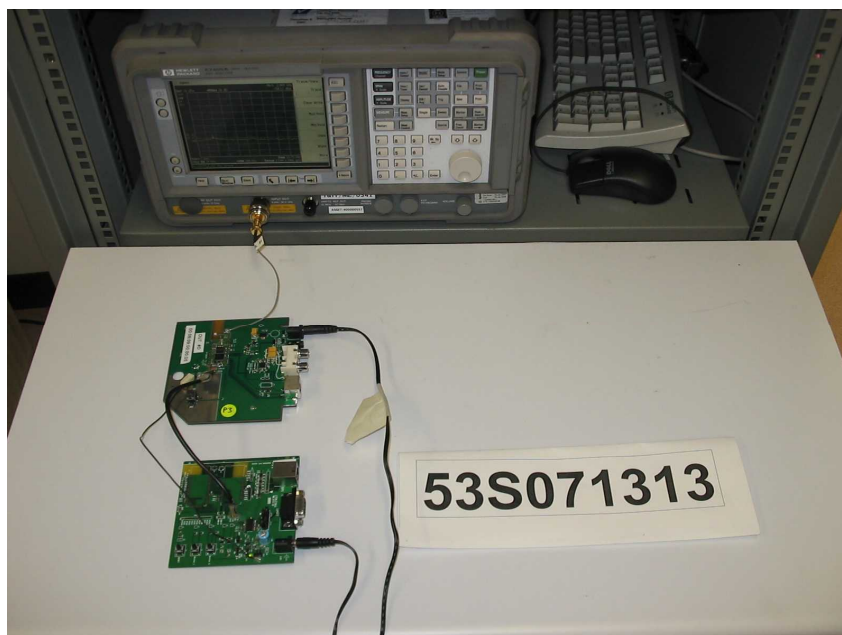
Spectrum Bandwidth (20dB Bandwidth Measurement) Test Setup
