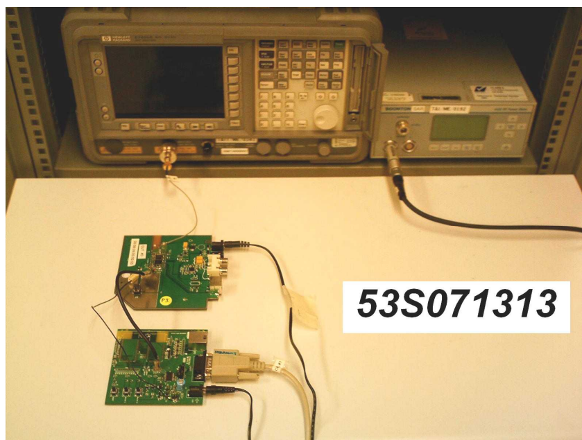
Number of Hopping Frequencies Test Setup
