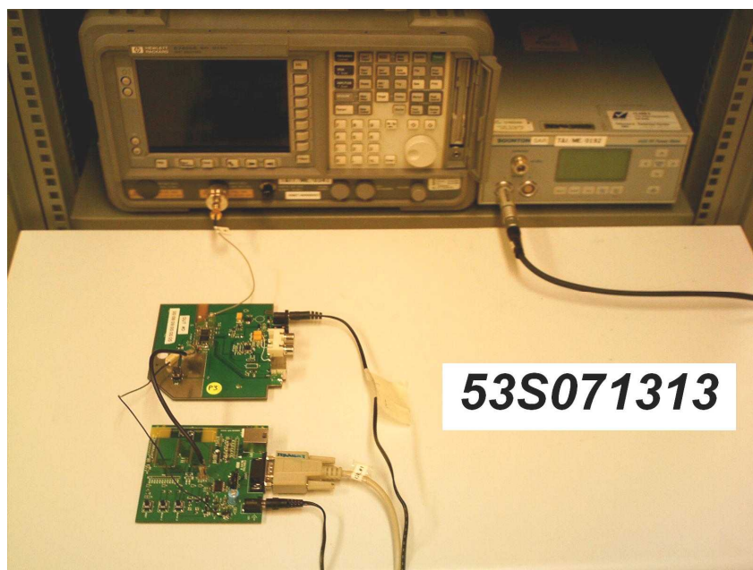
Peak Power Spectral Density Test Setup
