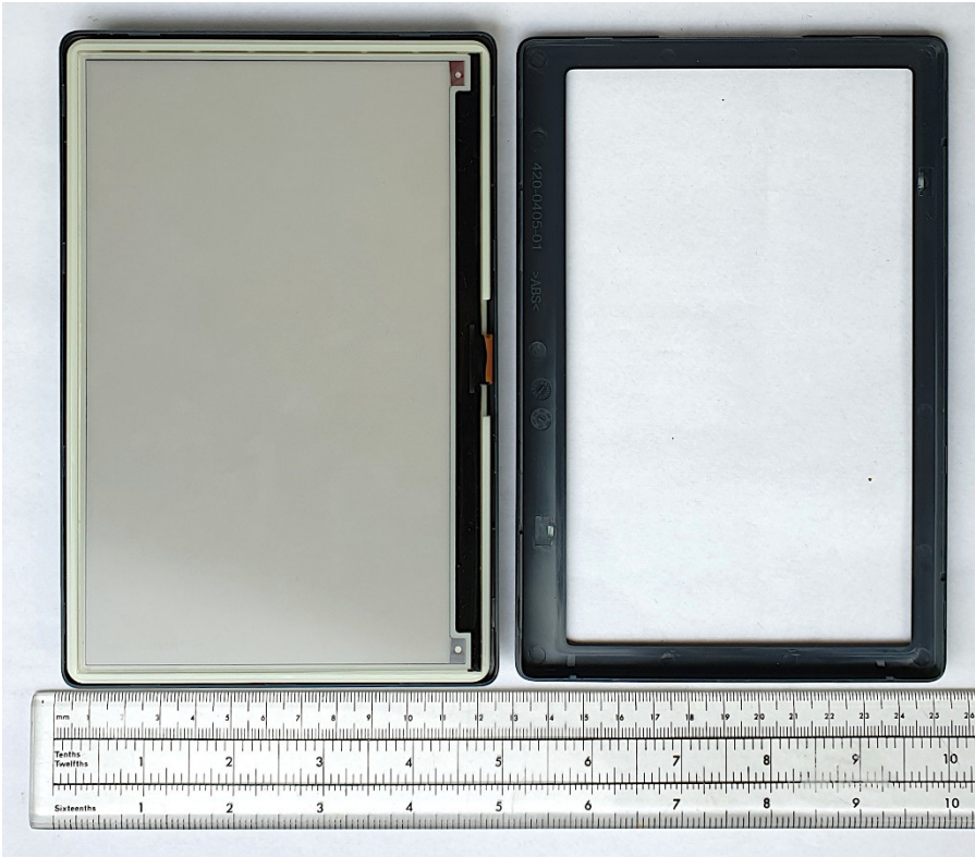
DD74-3A (Chroma Aeon 74) – Front View, with Front Cover removed.
