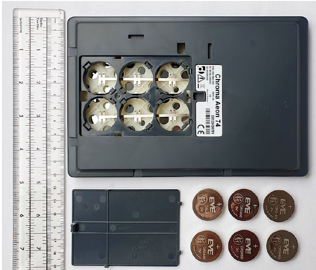
DD74-3A (Chroma Aeon 74) – Rear View, Battery Cover and Coin cells removed.
