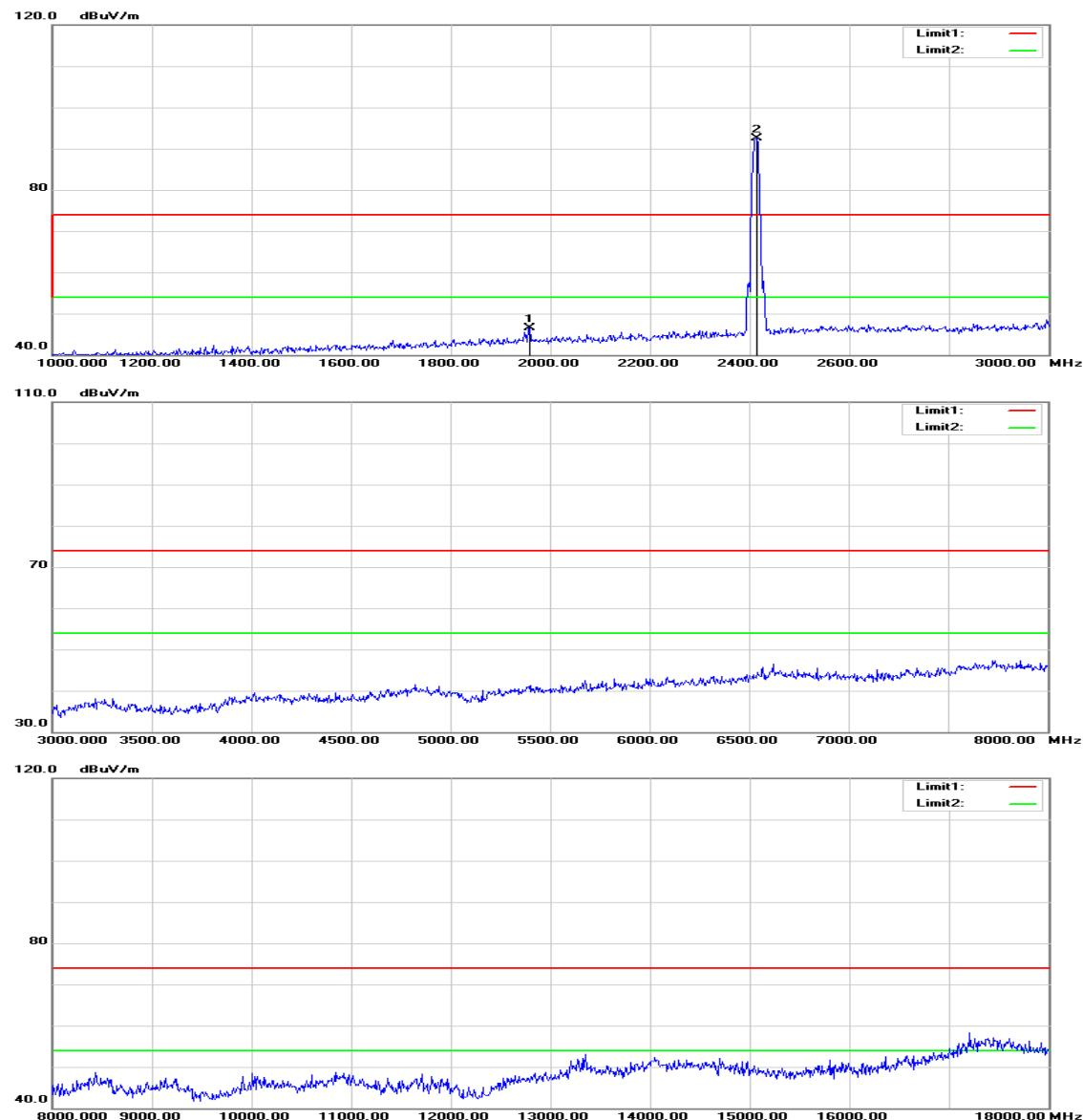
**Above 1 GHz****Operation Mode:** TX / IEEE 802.11b / CH Low**Test Date:** April 24, 2015**Temperature:** 27°C**Tested by:** Andy Shi**Humidity:** 53 % RH**Polarity:** Ver. / Hor.
