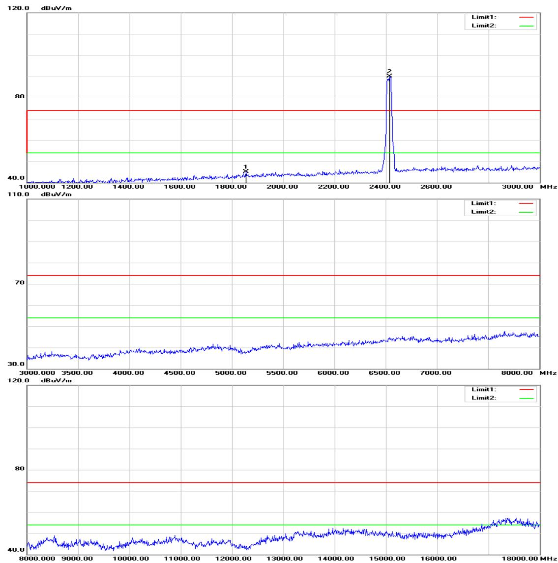
**Operation Mode:** TX / IEEE 802.11g / CH Low**Test Date:** April 24, 2015**Temperature:** 27°C**Tested by:** Andy Shi**Humidity:** 53 % RH**Polarity:** Ver. / Hor.
