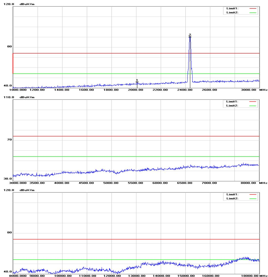
**Operation Mode:** TX / IEEE 802.11b / CH Mid**Test Date:** April 24, 2015**Temperature:** 27°C**Tested by:** Andy Shi**Humidity:** 53 % RH**Polarity:** Ver. / Hor.
