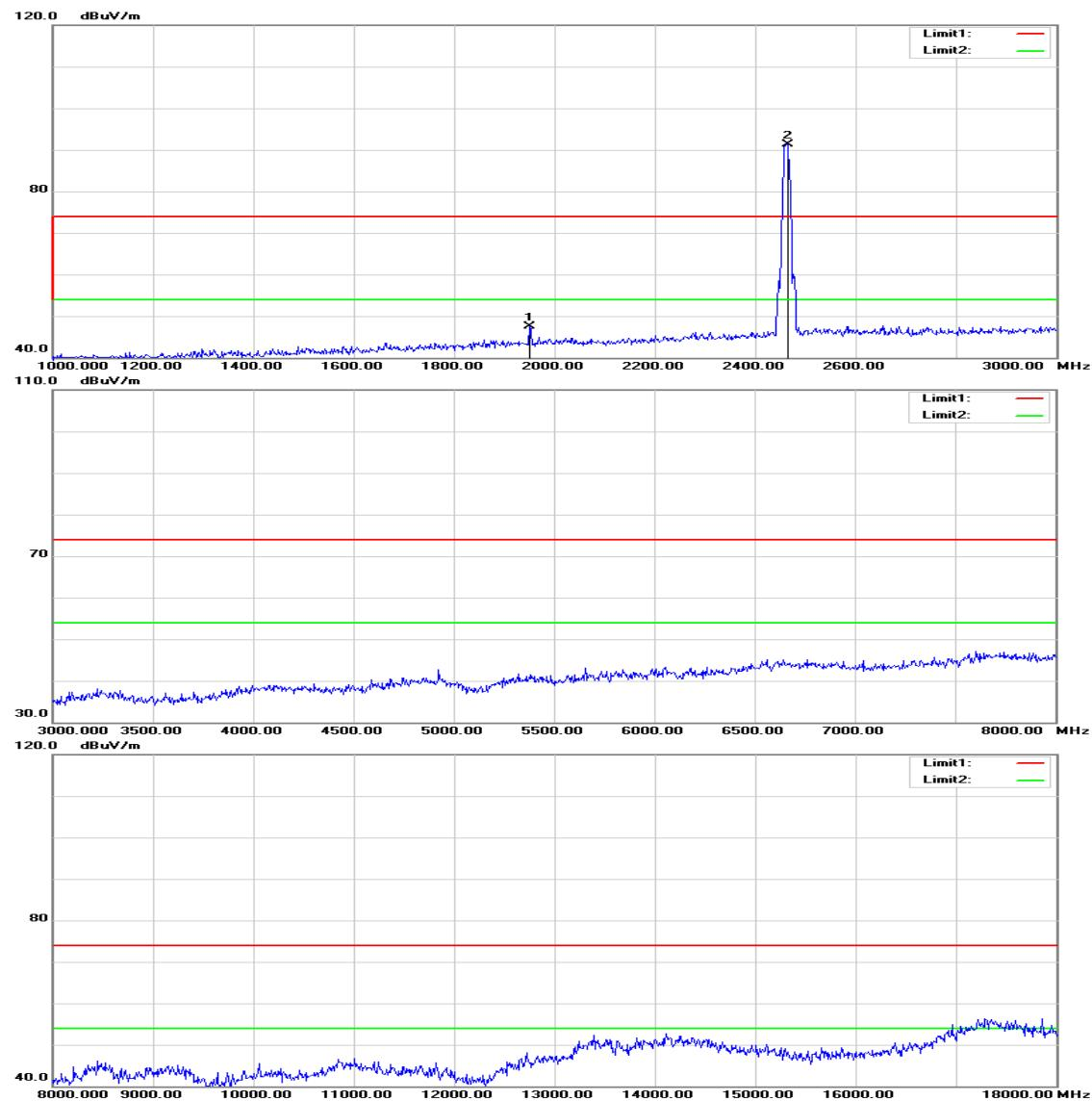
**Operation Mode:** TX / IEEE 802.11b / CH High**Test Date:** April 24, 2015**Temperature:** 27°C**Tested by:** Andy Shi**Humidity:** 53 % RH**Polarity:** Ver. / Hor.
