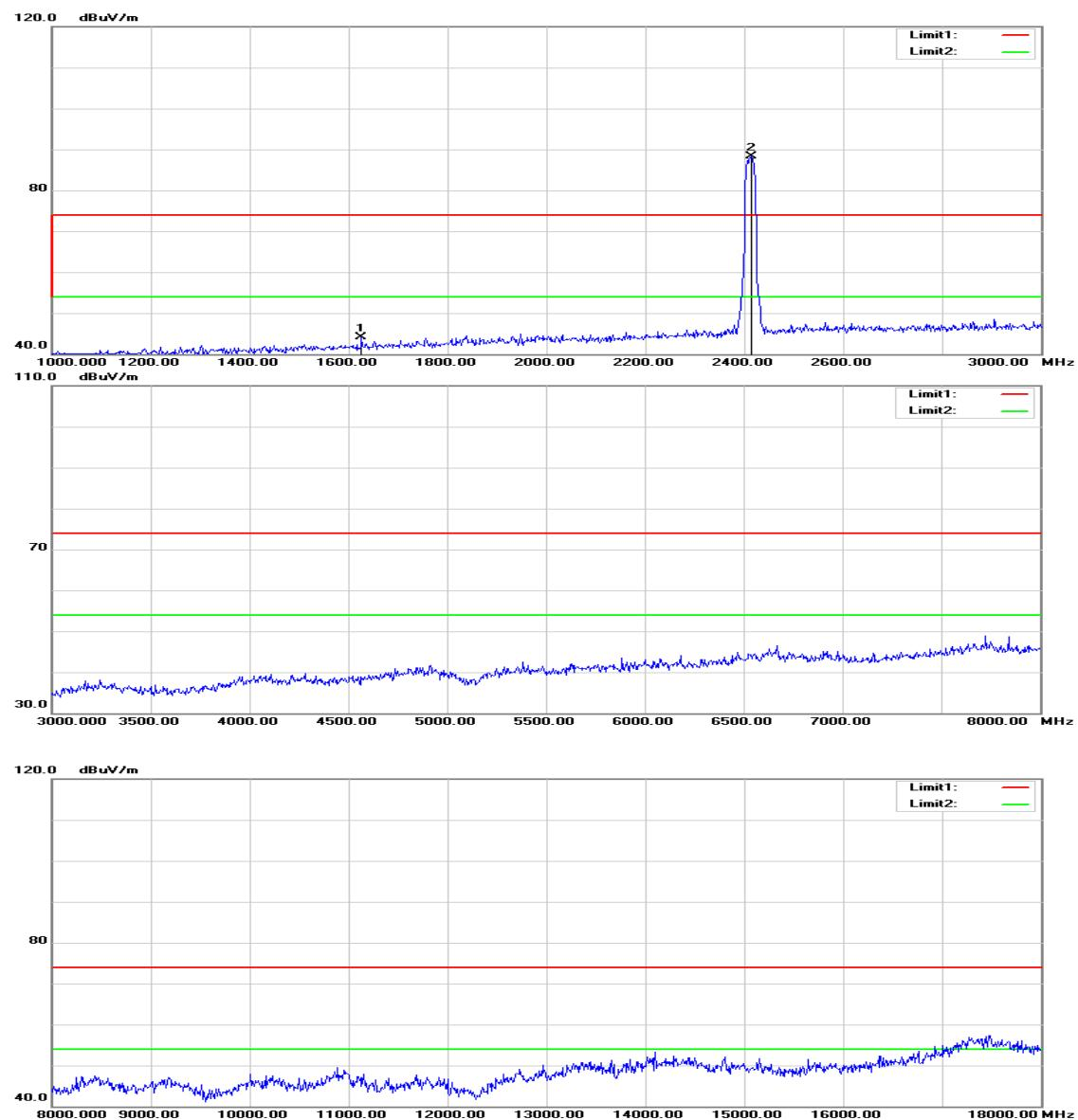
**Operation Mode:** TX / IEEE 802.11n HT 20 MHz mode Channel mode / CH Low **Test Date:** April 24, 2015
