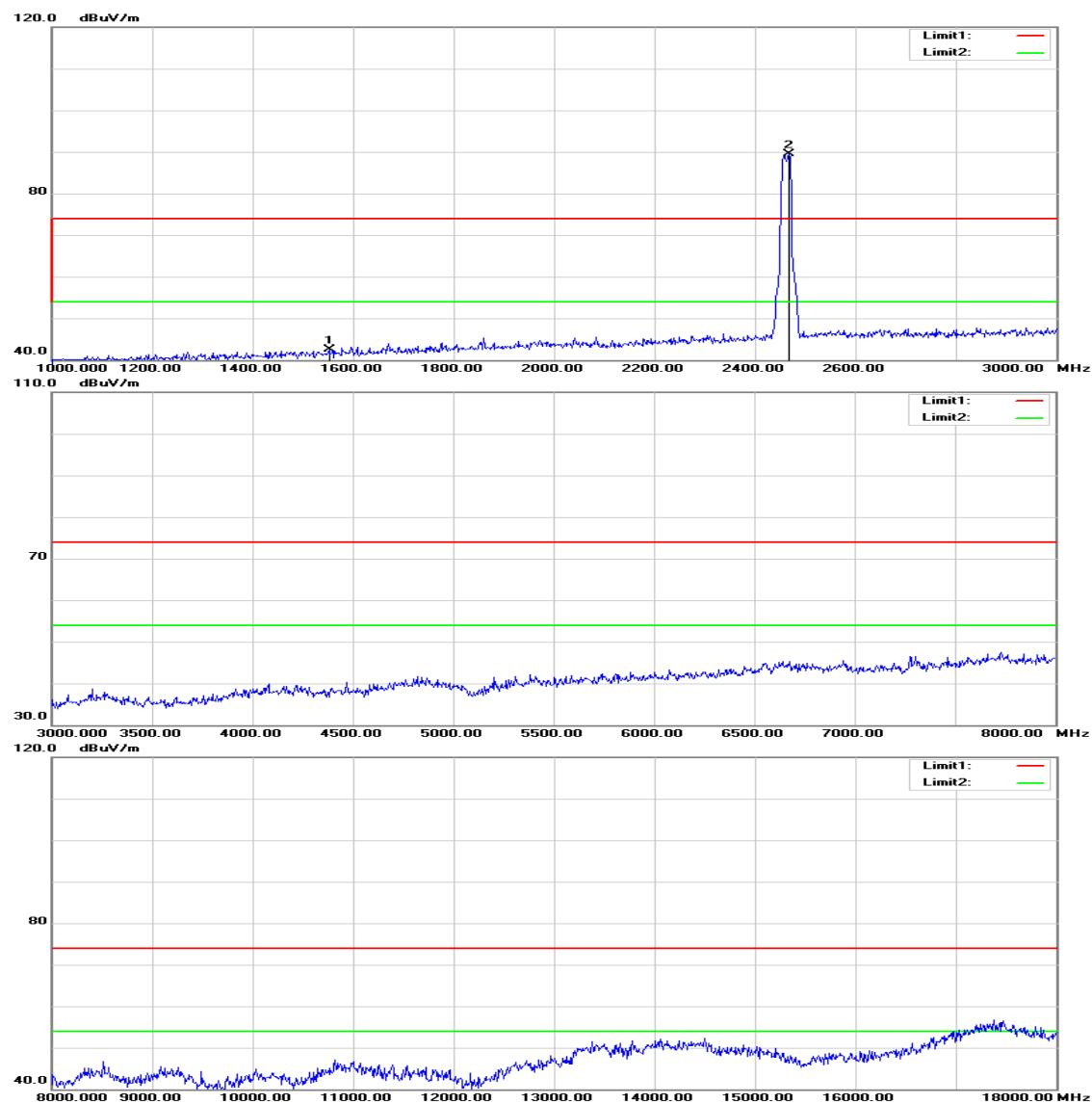
**Operation Mode:** TX / IEEE 802.11g / CH High**Test Date:** April 24, 2015**Temperature:** 27°C**Tested by:** Andy Shi**Humidity:** 53 % RH**Polarity:** Ver. / Hor.
