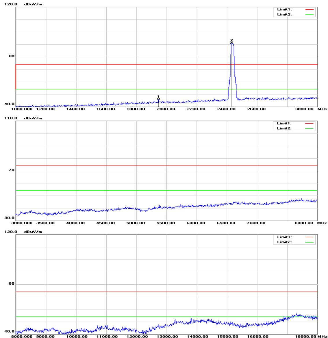
**Operation Mode:** TX / IEEE 802.11n HT 20 MHz mode / CH Mid
