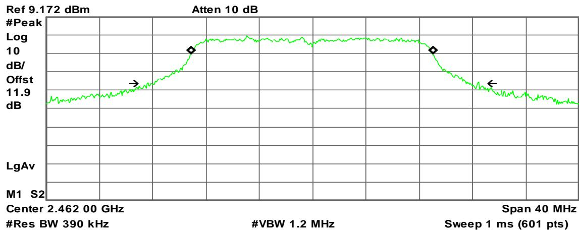
**Occupied Bandwidth****18.1689 MHz**Transmit Freq Error
