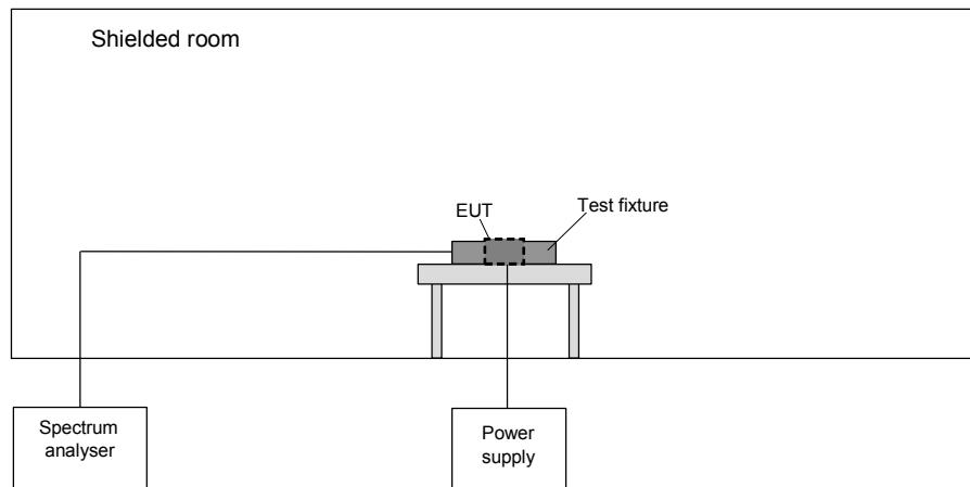
The following procedure will be used for the spectrum mask measurement:
