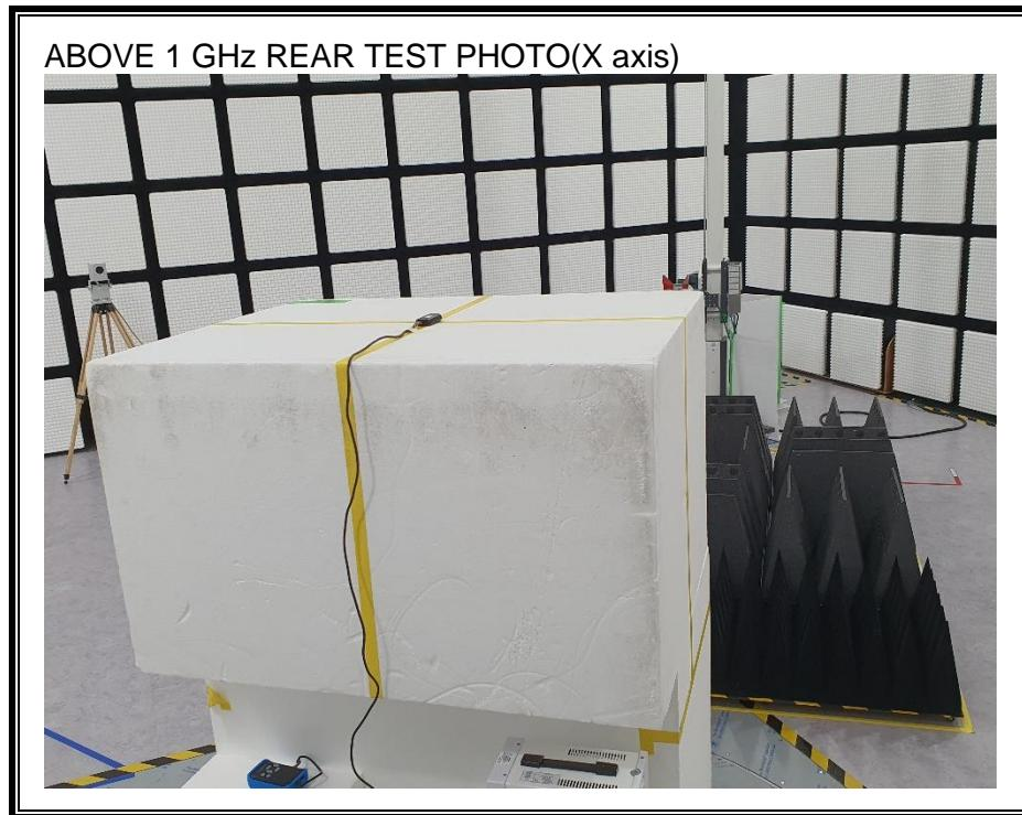
3) RADIATED RF MEASUREMENT SET-UP (Axis)
