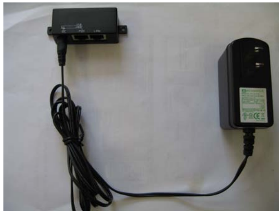
Figure #8: POE and AC/DC converter
