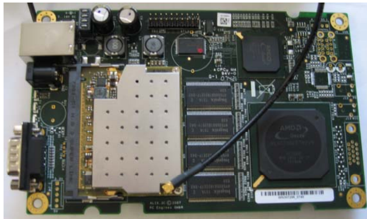
Figure #6: PMX 3.0 Internal Configuration (bottom view of circuit board)
