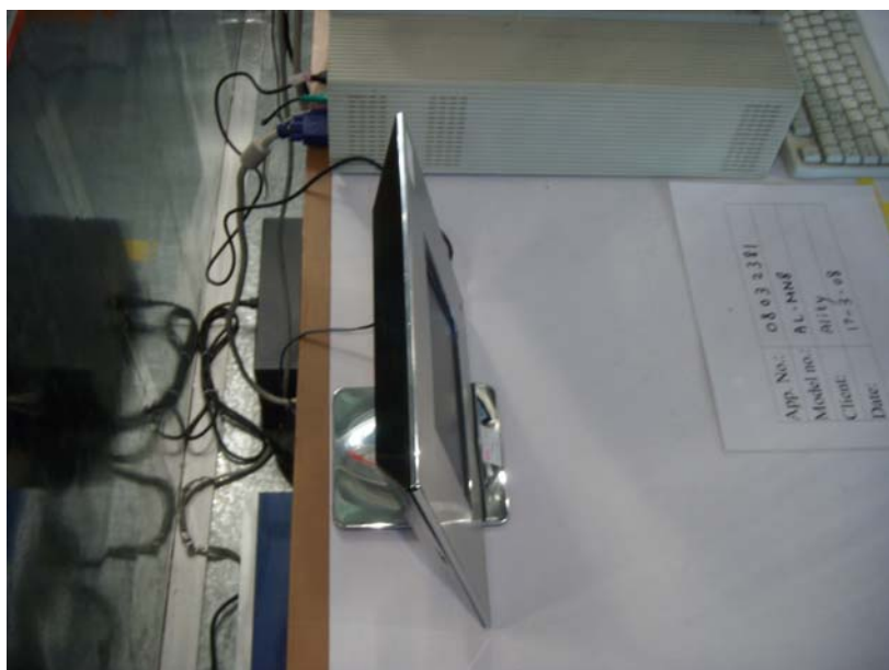
Measurement of Conducted Emission Test Set up
