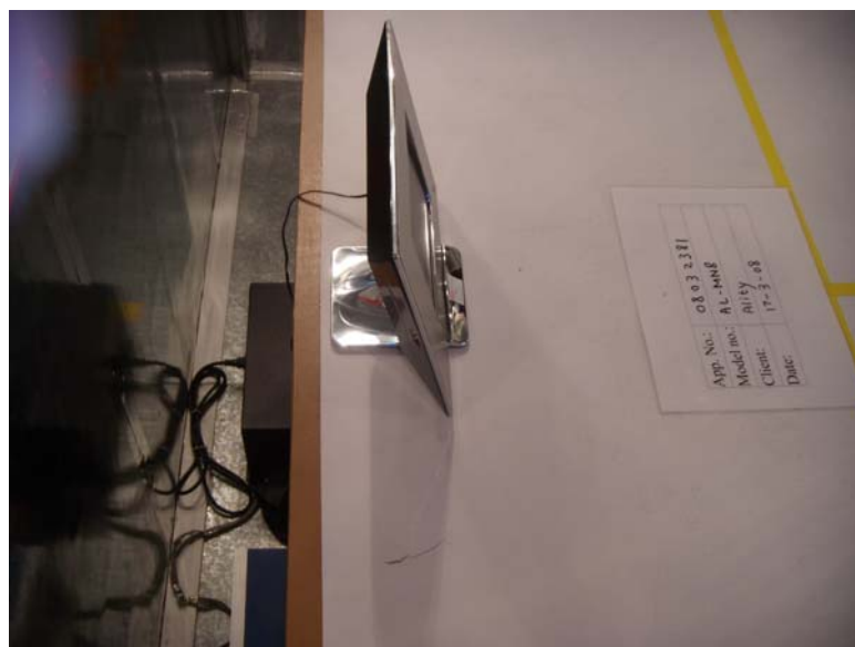
Measurement of Conducted Emission Test Set up
