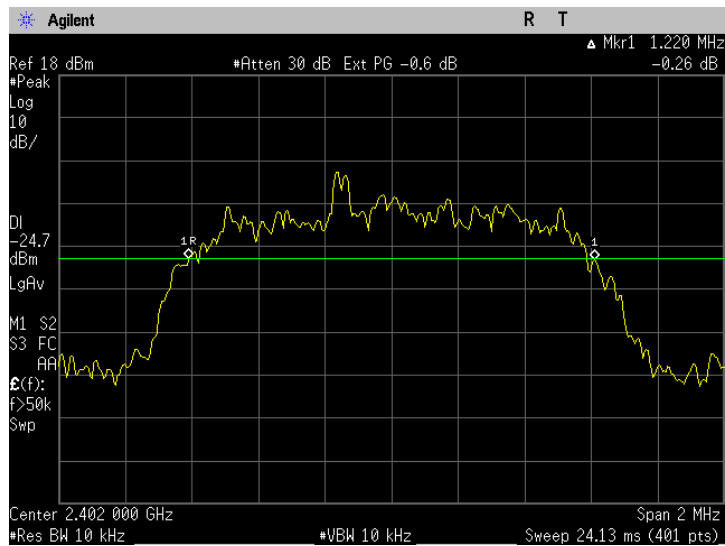
Figure 6-1b: 20dB Bandwidth EDR DQPSK, Channel 0.
