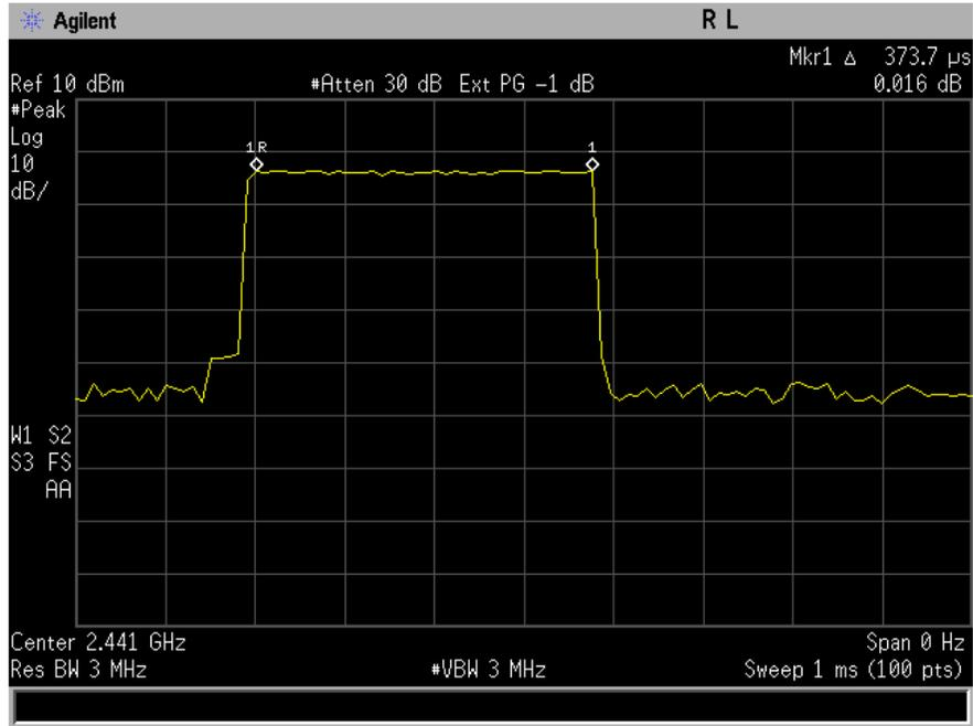
**Figure 9: Duration of one transmission (Channel 39).**
