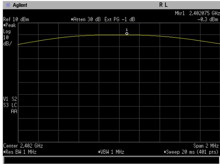
**Figure 5-1: Peak Output Power, Basic Rate Channel 0.**
