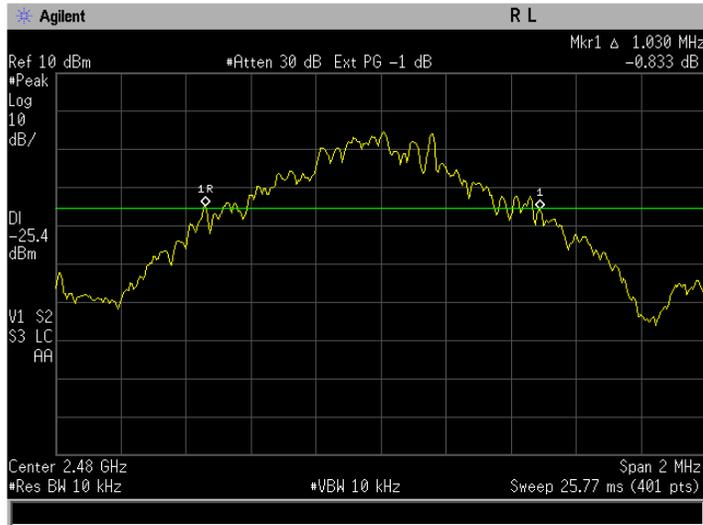
**Figure 6-3a: 20dB Bandwidth Basic rate, Channel 78.**
