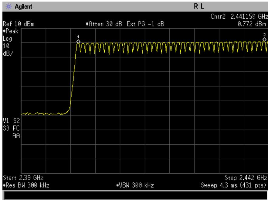
**Figure 8a: Number of Hopping Frequencies (Channels 0-39).**
