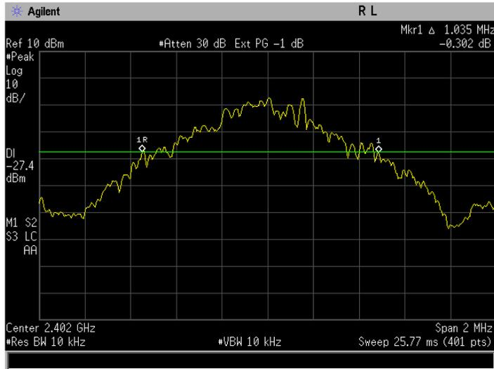
**Figure 6-1a: 20dB Bandwidth Basic rate, Channel 0.**
