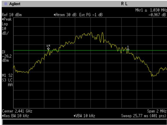
**Figure 6-2a: 20dB Bandwidth Basic rate, Channel 39.**
