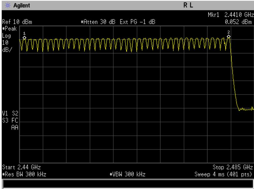
**Figure 8b: Number of Hopping Frequencies (Channels 39-78).**
