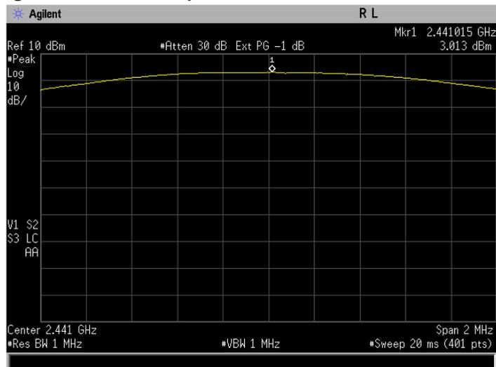
**Figure 5-2b: Peak Output Power, EDR D8PSK Channel 39.**
