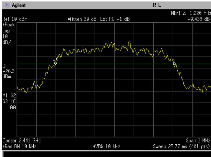
**Figure 6-2c: 20dB Bandwidth EDR D8PSK, Channel 39.**
