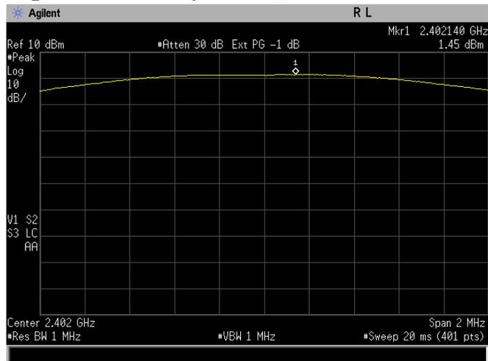
**Figure 5-1a: Peak Output Power, EDR DQPSK Channel 0.**
