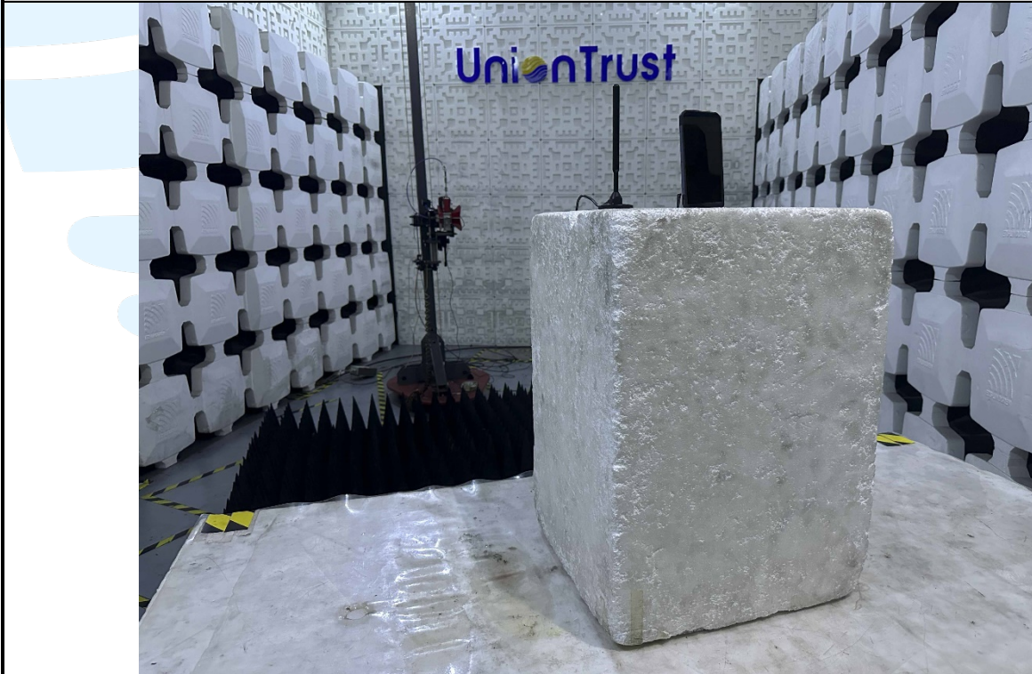
Radiated emission Test Setup (Above 1 GHz)
