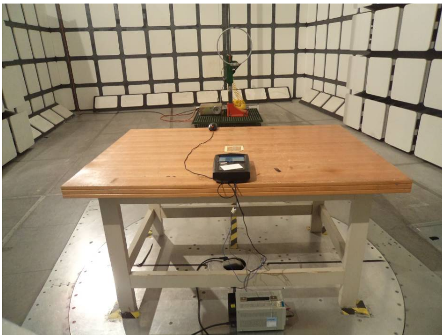
Radiated Emissions Back View (Below 30 MHz)
