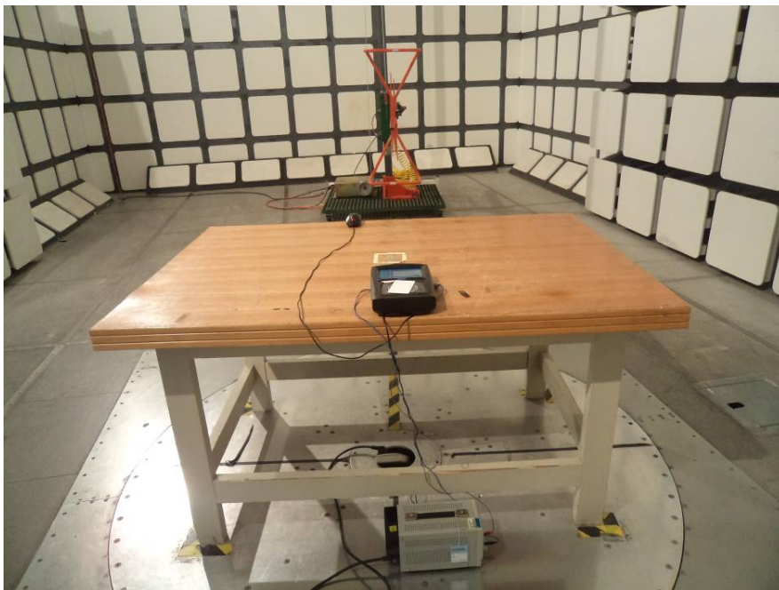
Radiated Emissions Back View (Above 30 MHz)
