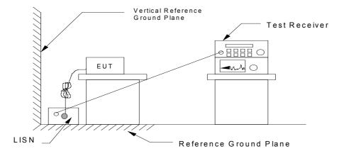
**Test Set-Up 4**
