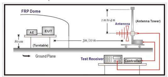
Above 1GHz Test Setup:
