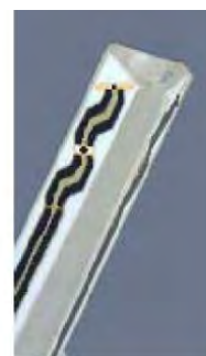
Figure E.2.2 Probe Thick-Film Technique
