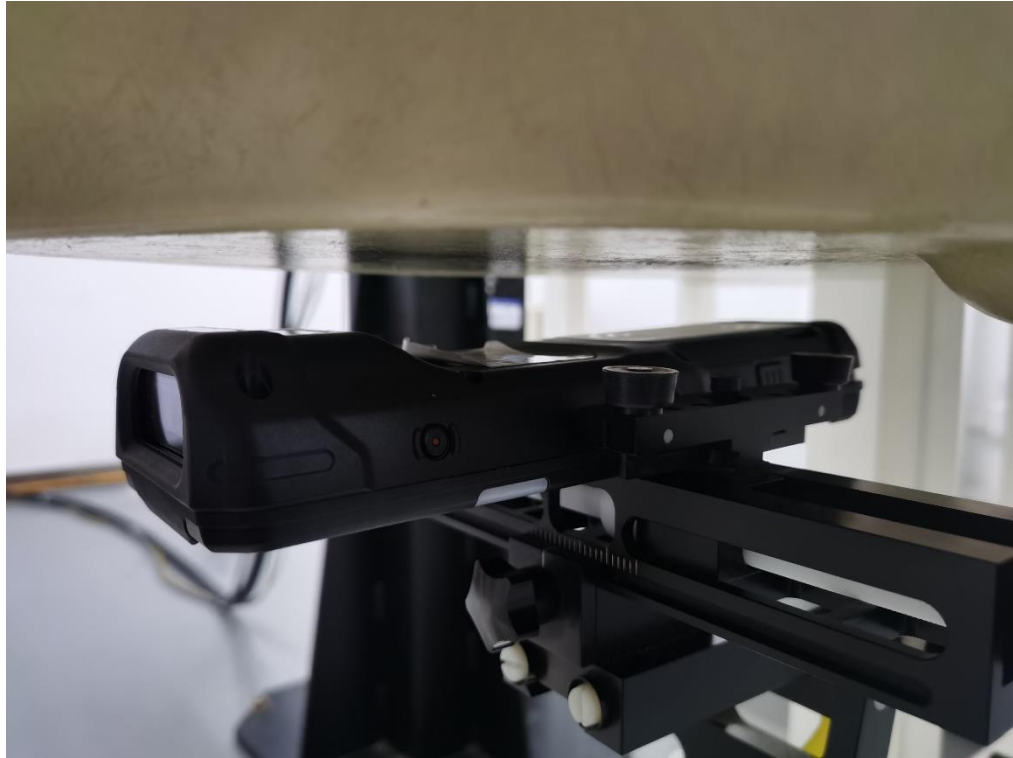
Picture 6: Rear Side with AE2 Battery (15mm)
