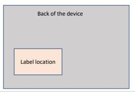
The label of device is located in the battery room. The label is visible to the users as they purchase the product and install the SIM card.
