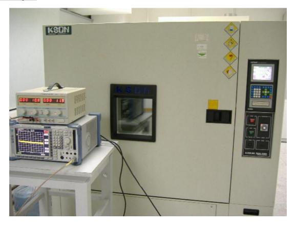
Effective Radiated Power & Occupied bandwidth & Unwanted Radiation
