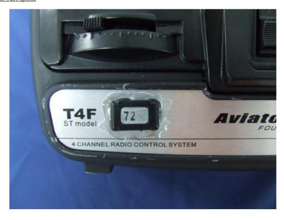
Crystal access panel is permanently glued shut in manufacturing.
