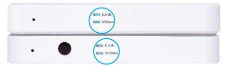
6. If the Sender and Receiver units do not pair automatically, point the IR remote at the IR sensor window on the Receiver and press Menu. Navigate through the on-screen menu and have the Receiver look for a Sender. Using a paper clip, press and hold the pairing button on the Sender until the Link LED stops blinking. Press OK on the remote. A message indicating that the Sender and the Receiver have been paired will appear on the display.
