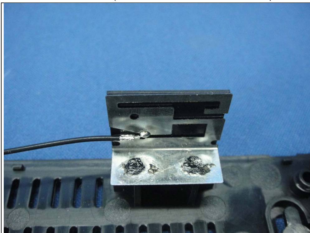
WIFI Antenna 1 (Model No.: RFA-25-G170-70B-154)
