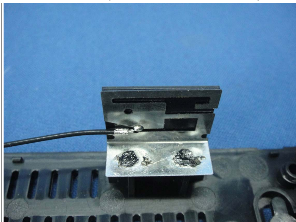
WIFI Antenna 2 (Model No.: RFA-25-G170-70B-154)
