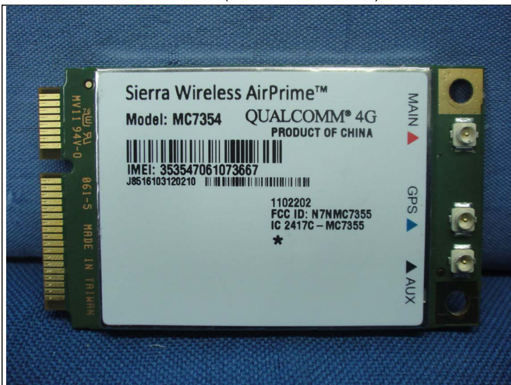
3G module (Model No.: MC7354)
