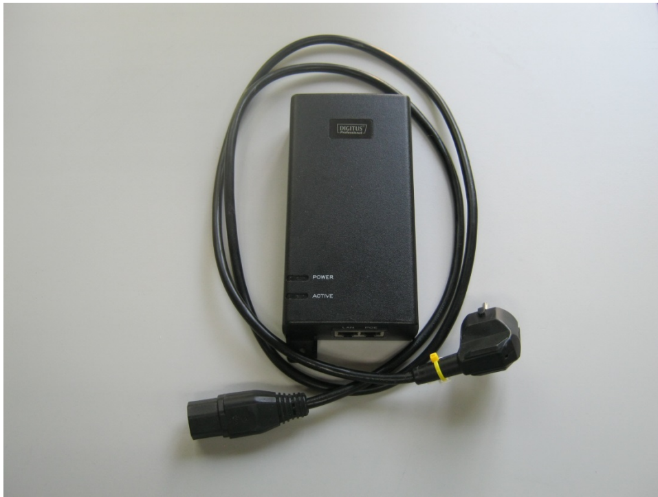
Photograph A3-3: Power over Ethernet injector
