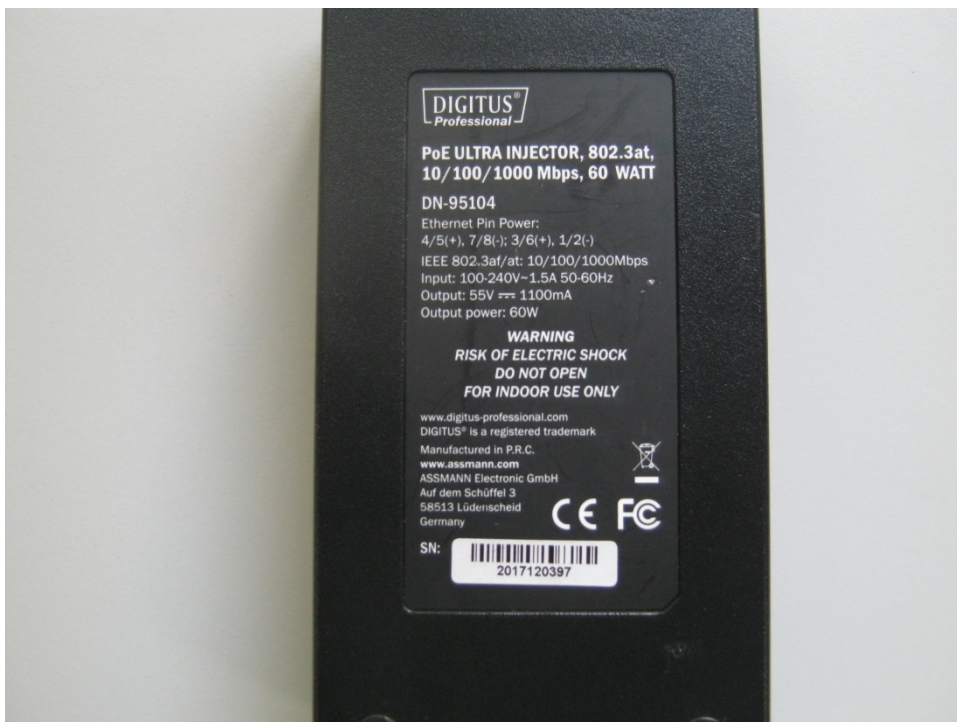
Photograph A3-4: Label of Power over Ethernet injector
