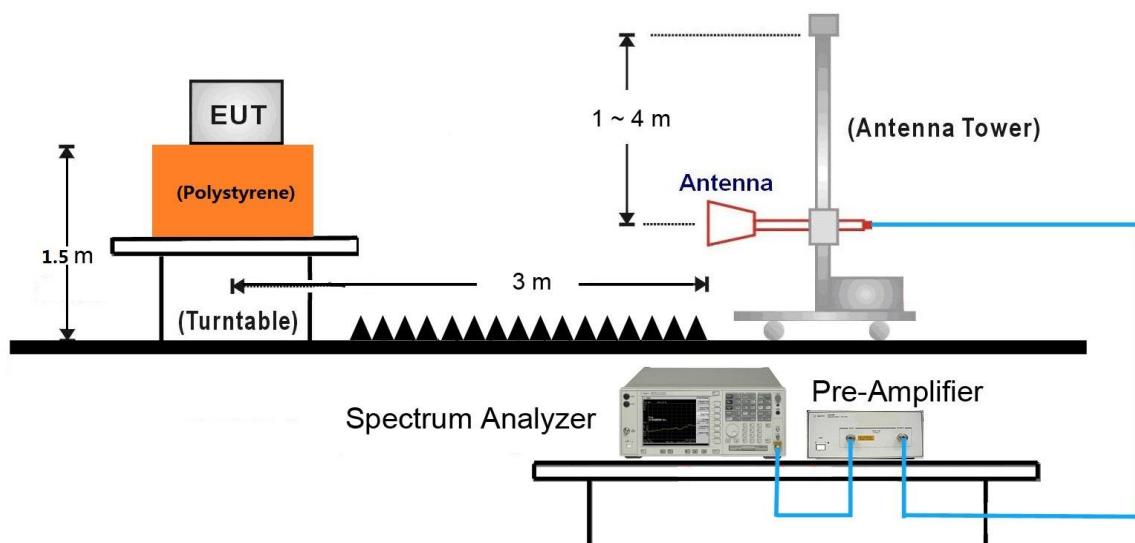
18GHz ~25GHz Test Setup:
