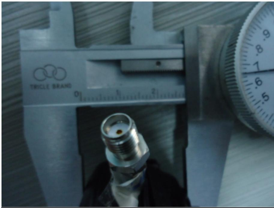
The thickness of EUT is about 28mm. The chip antenna is assembled on the PCB. The main PCB is assembled on the middle of the EUT. So the separation distances are about 14mm. According to the Appendix A of the KDB 447498. The limit of SAR test exclusion is at least 19mW.
