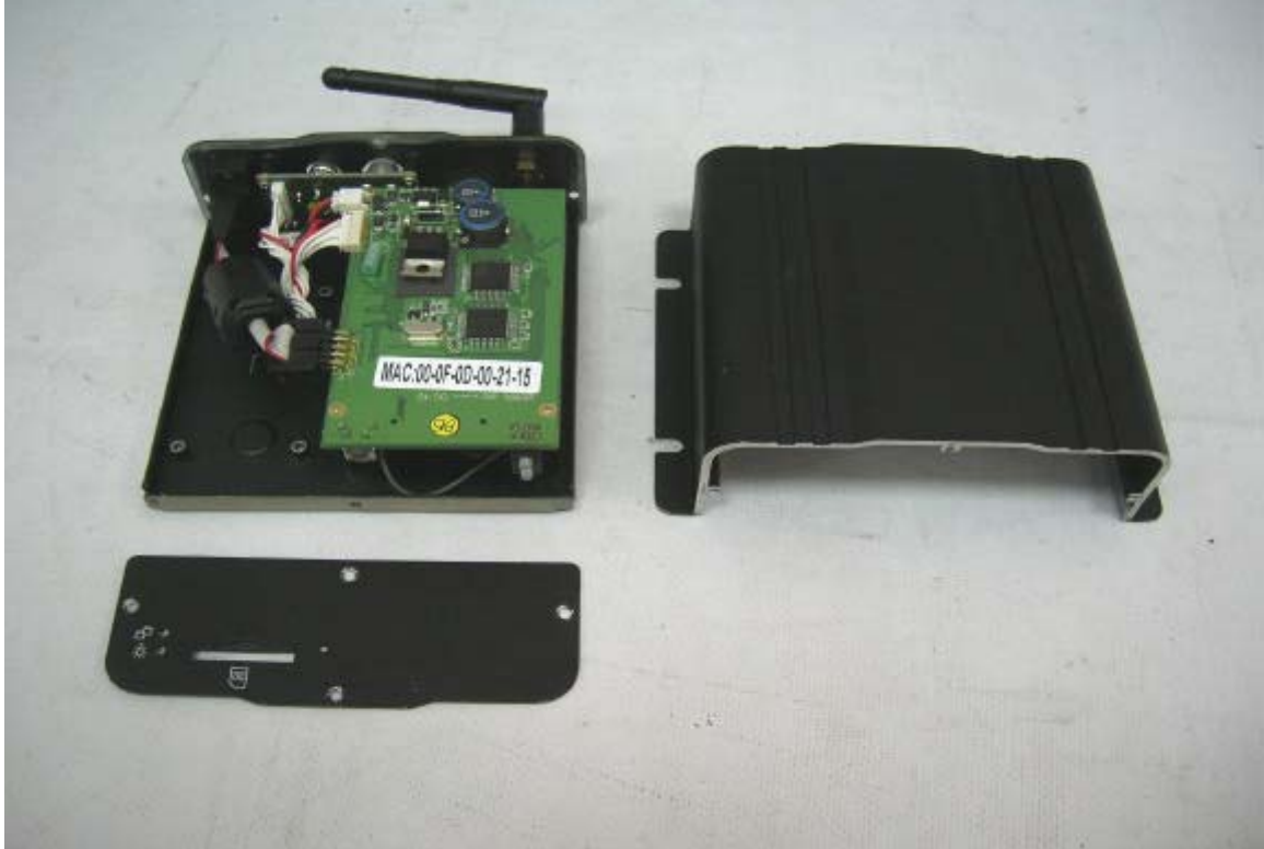
PHOTO. 4. EUT COMPONENT VIEW
