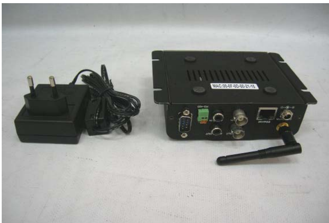
PHOTO. 2. EUT REAR VIEW
