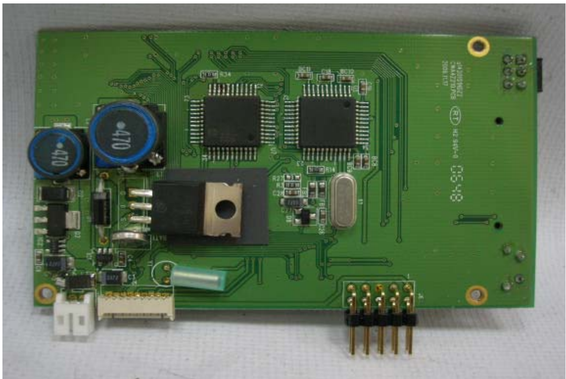
PHOTO. 4. EUT COMPONENT VIEW
