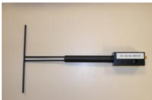
Figure 1 – Satimo COMOSAR Validation Dipole
