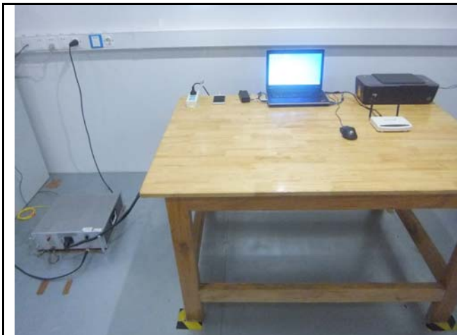
Conducted Emissions Test Setup – Front View
