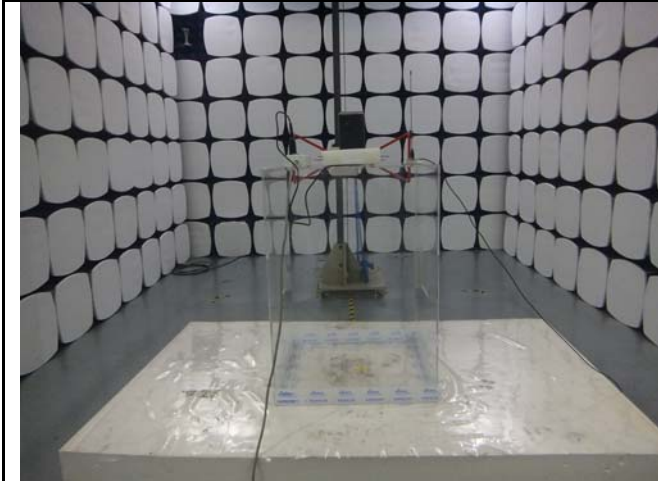
Radiated Spurious Emissions Test Setup Below 1GHz
