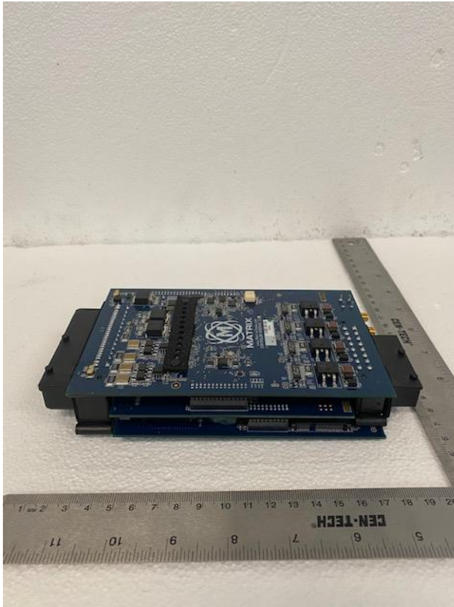
Figure 1. Processor PCB, Wireless PCB and Interface PCB Stacked Assembly
