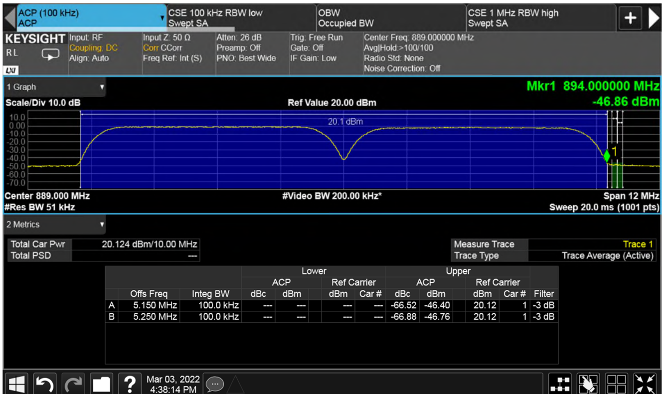
Plot of upper band edge for High channels (886.5 & 891.5 MHz)
