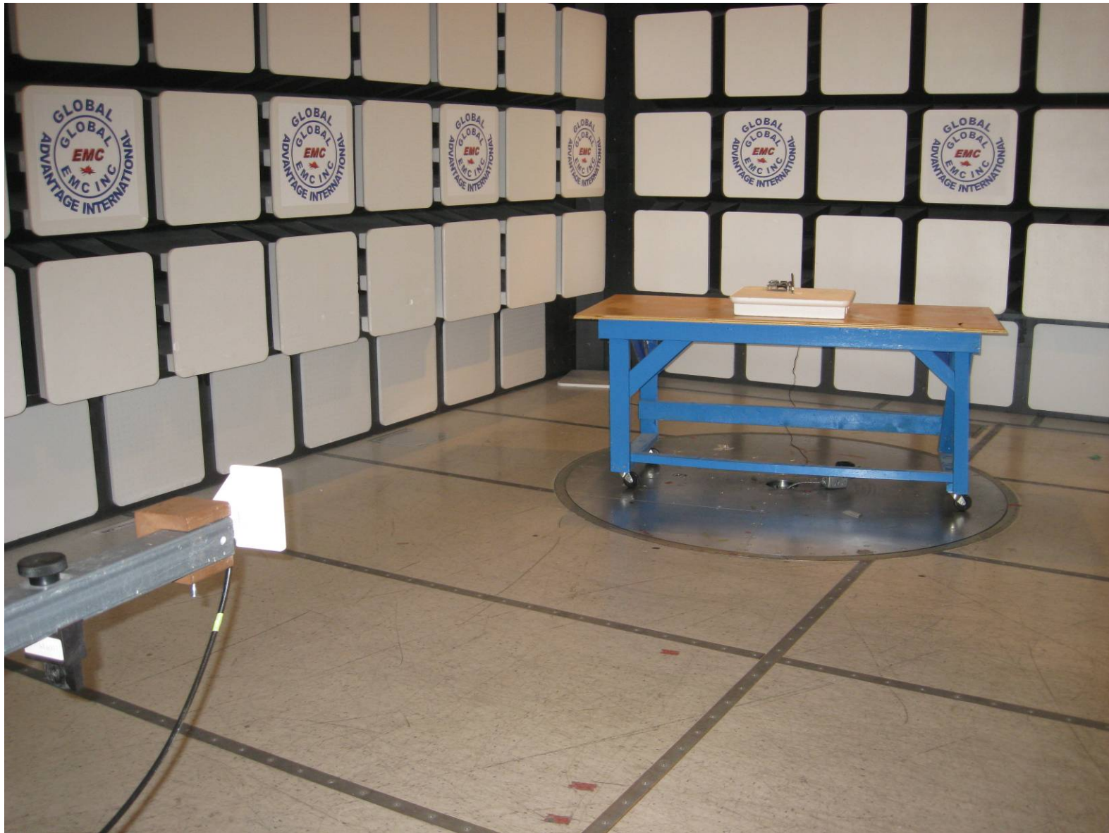
Radiated Emissions Setup Photo 2
