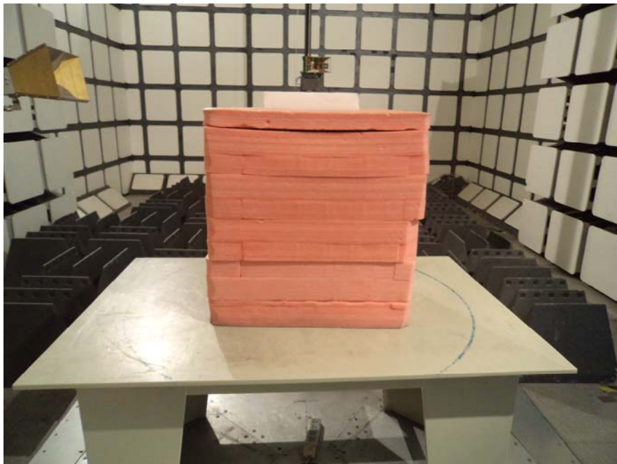
Radiated Emissions Test View (Above 1 GHz)
