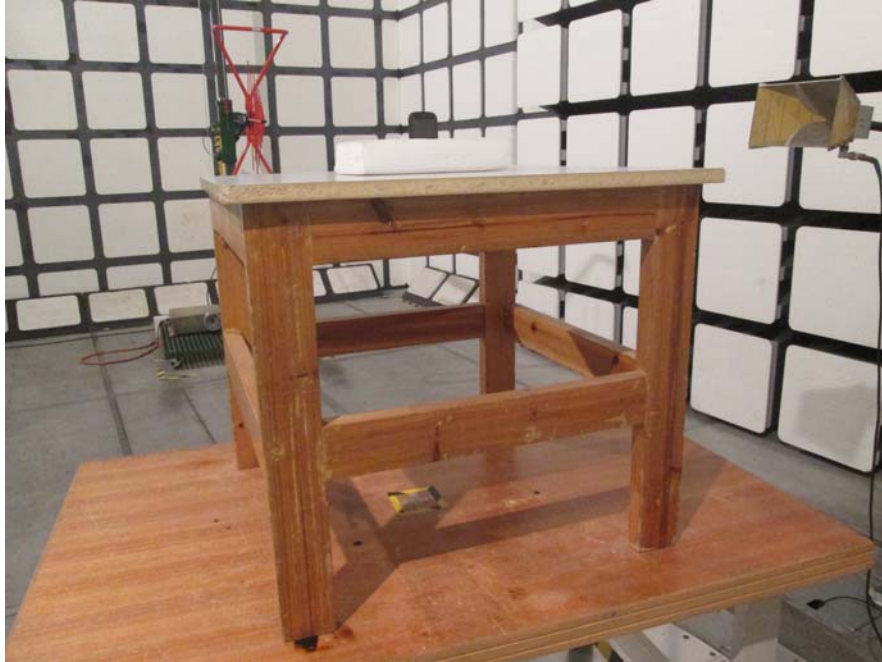
Radiated Emissions Test View (Below 1 GHz)
