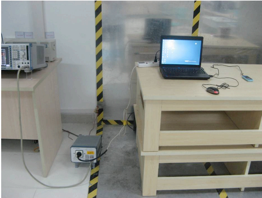
FCC LINE CONDUCTED EMISSION TEST SETUP
