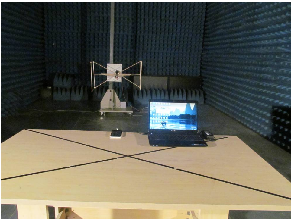
FCC RADIATED EMISSION TEST SETUP
