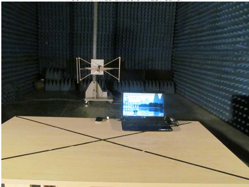
FCC RADIATED EMISSION TEST SETUP
