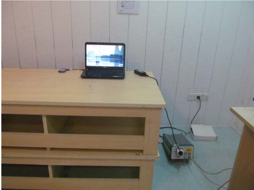
FCC LINE CONDUCTED EMISSION TEST SETUP
