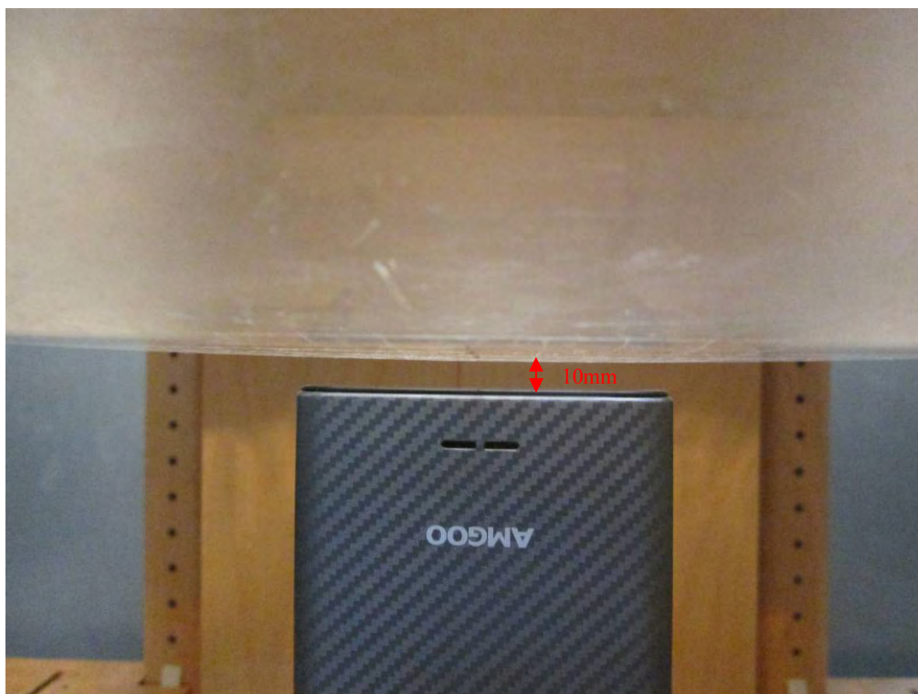
Body-worn Bottom Setup Photo (10mm)
