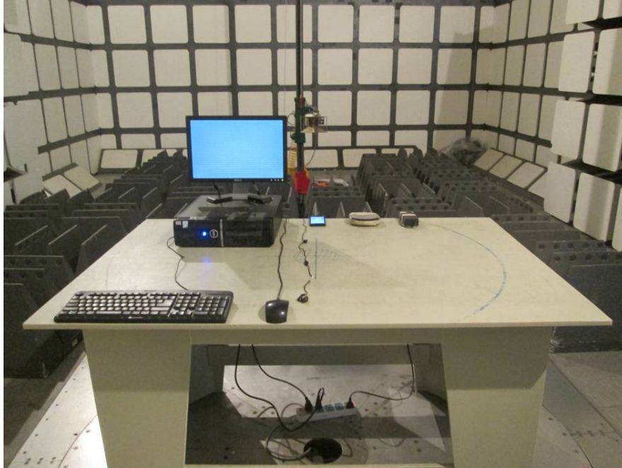
Radiated Emissions – Front View (Above 1 GHz)
