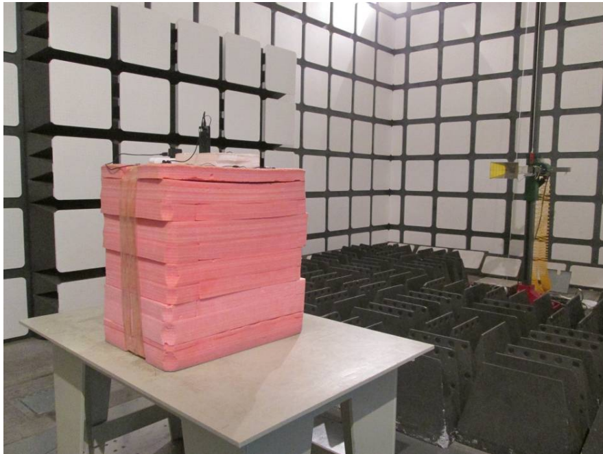
Radiated Emissions View (Above 1 GHz)
