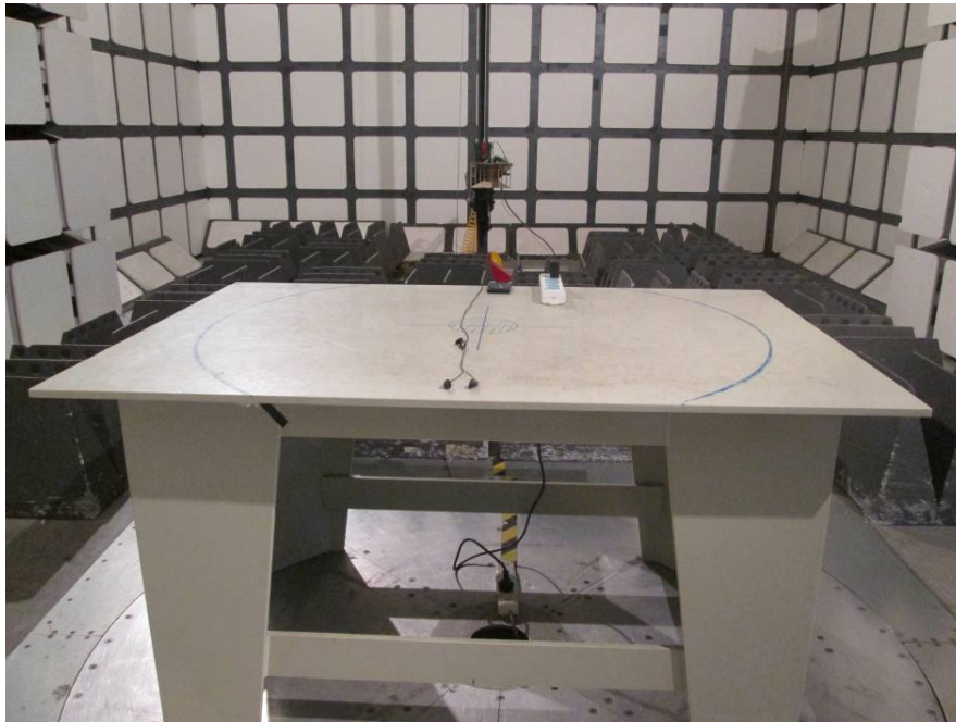
Radiated Emissions Front View (Above 1GHz)
