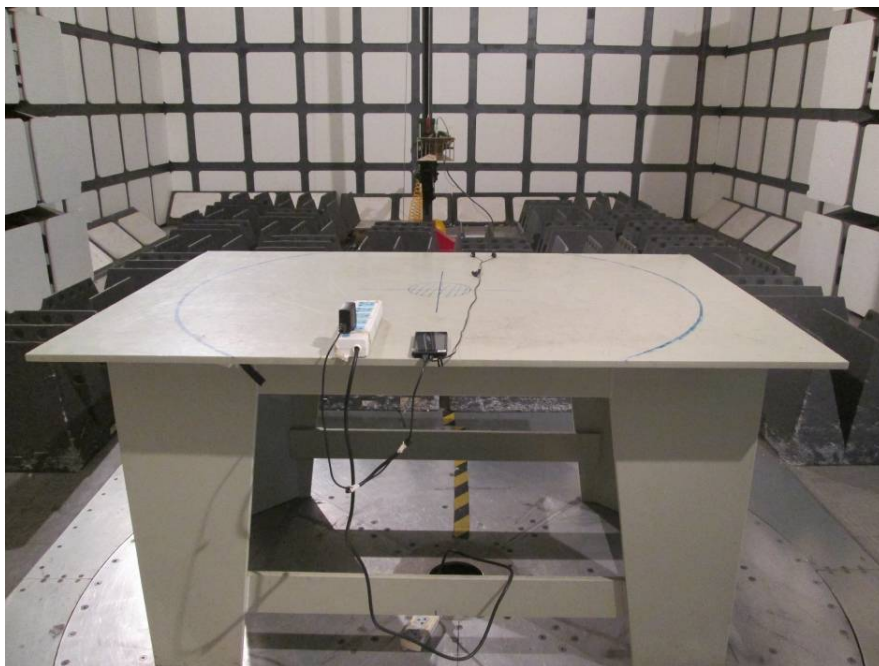
Radiated Emissions Rear View (Above 1GHz)
