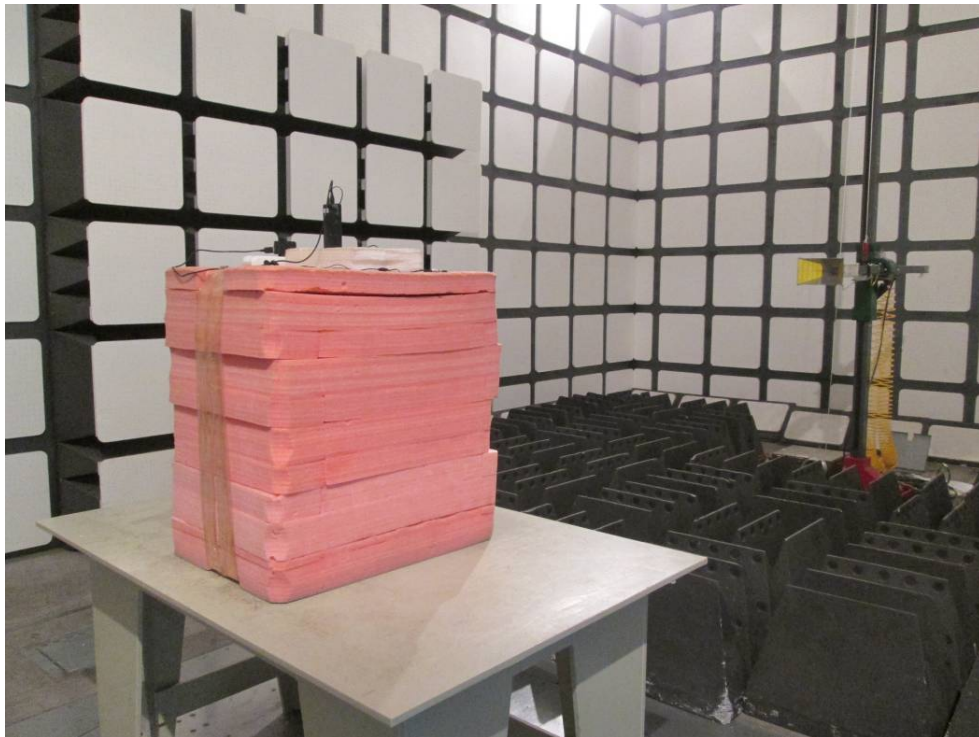
Radiated Emissions View - (Above 1 GHz)
