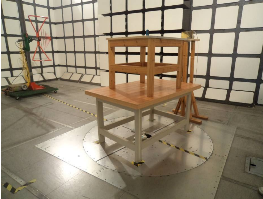
Radiated Emissions Test View (Below 1 GHz)
