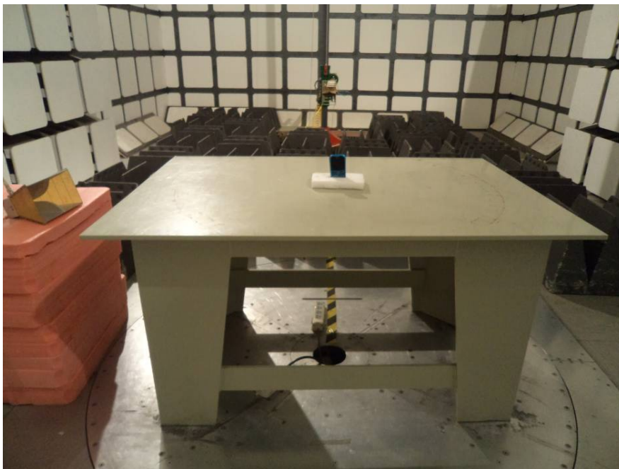
Radiated Emissions View (Above 1 GHz)
