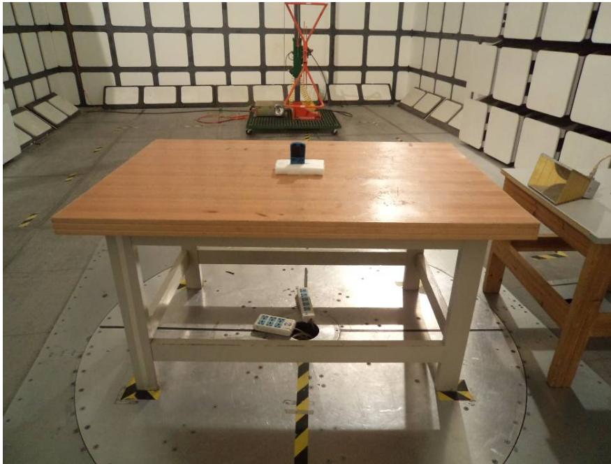
Radiated Emissions View (Below 1 GHz)
