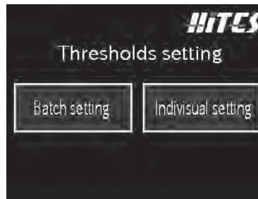
Management values for yellow and red can be set for tire air pressure and air temperature inside tire of all positions (including spare tire).
