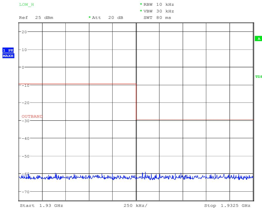
**Out-of-band Unwanted Emissions: CH F<sub>L</sub>.**
