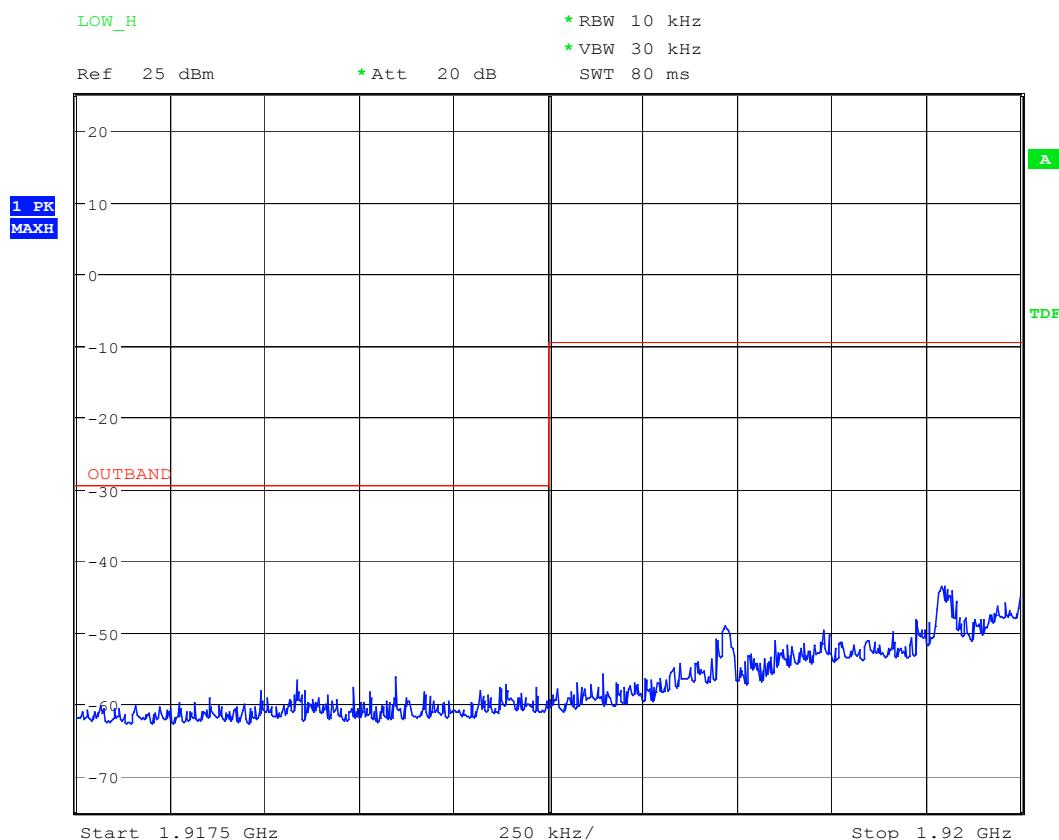
**Out-of-band Unwanted Emissions: CH F<sub>L</sub>.**
