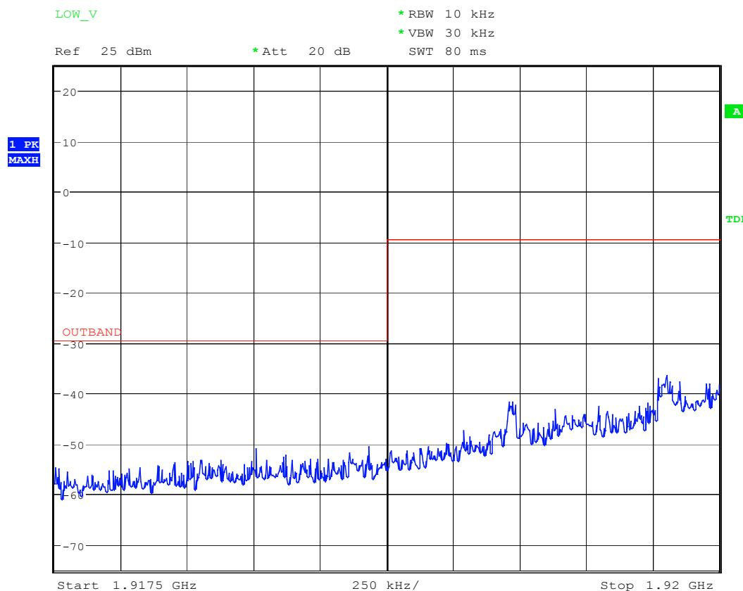
**Out-of-band Unwanted Emissions: CH F<sub>L</sub>.**
