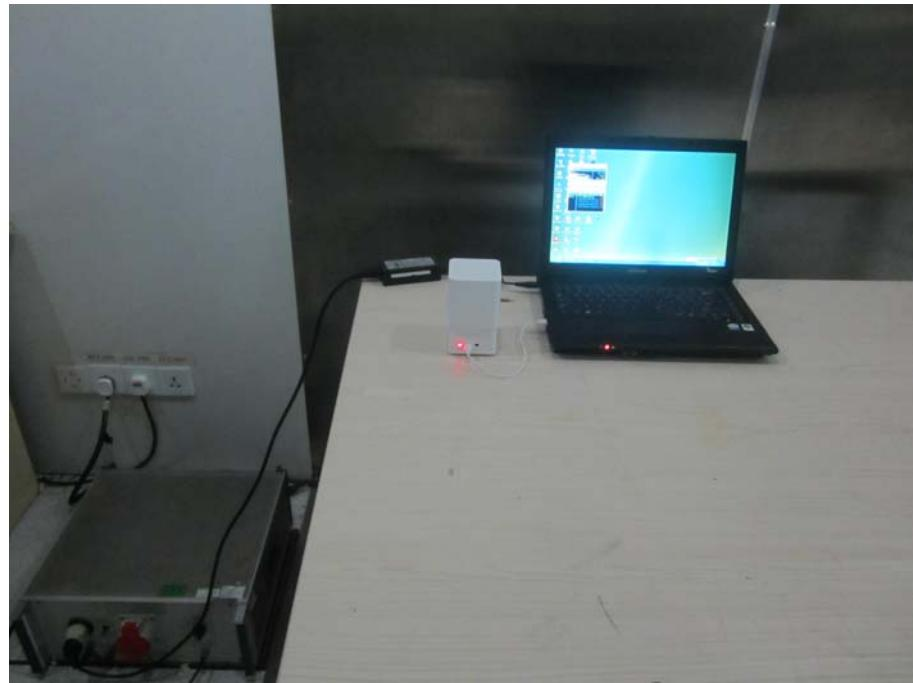
Radiation Emission Test Setup (9KHz to 30MHz)
