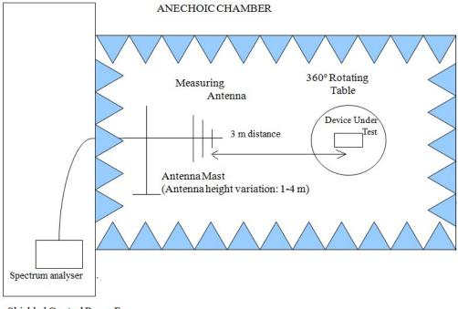
Shielded Control Room For Radiated Measurements
