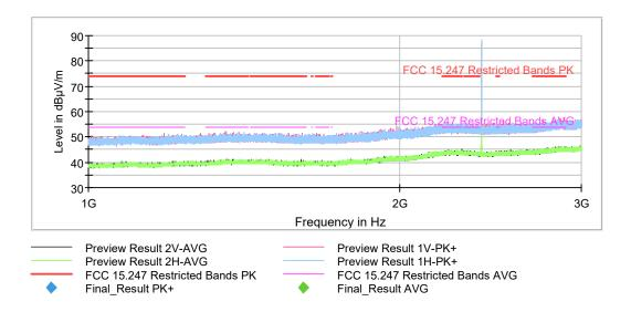
The highest peak is the carrier frequency (Bluetooth LE 2402 MHz)
