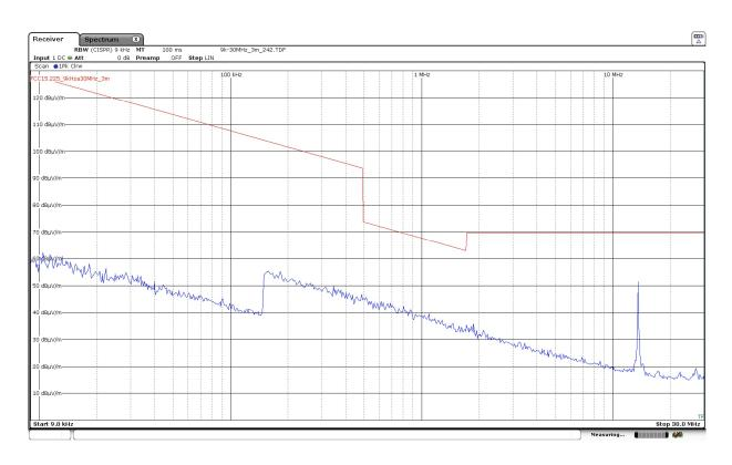
The highest peak is the carrier frequency (RFID 13.56 MHz)
