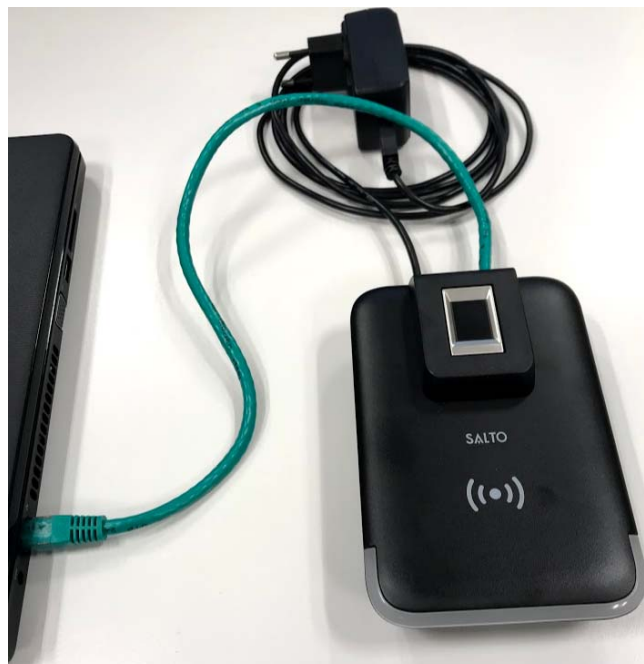
Photo 6: Ethernet connection + Power supply
