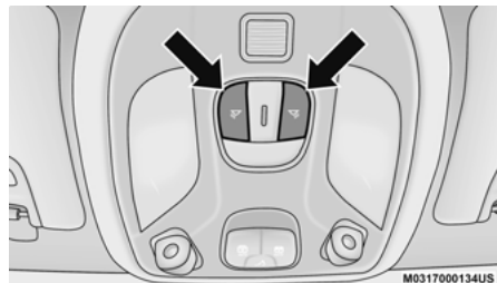
Overhead Light Switches
