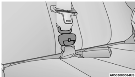
Inserting Mini-Latch Plate Into Mini-Buckle
