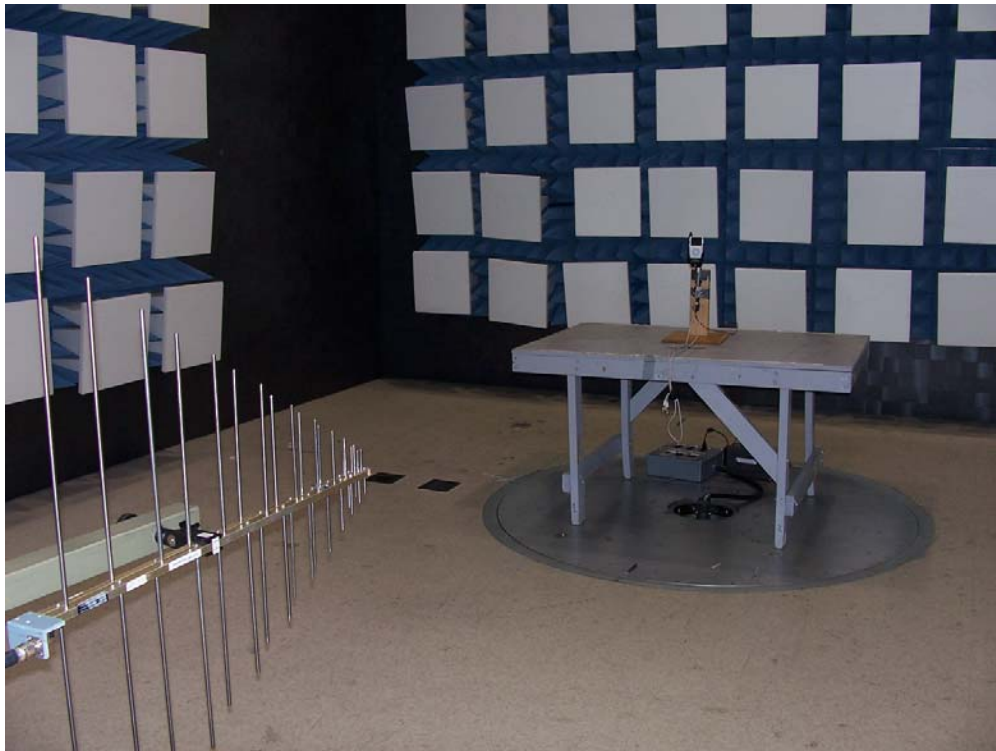
Figure 7 - Photo of Part 15.239 testing set up (Front)
