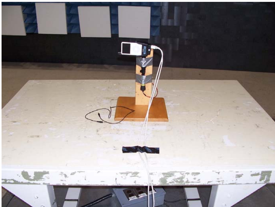
Figure 12 – Shows one of the 3 orthogonal positions used for testing.
