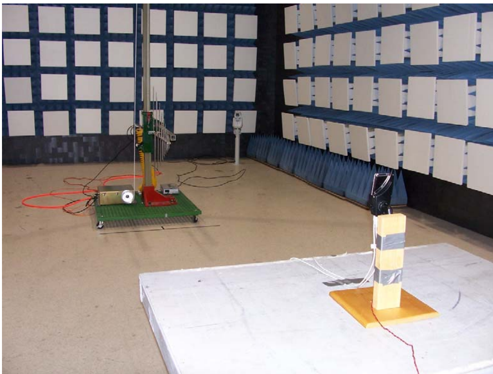
Figure 8 - Photo of Part 15.209 testing set up (Back)
