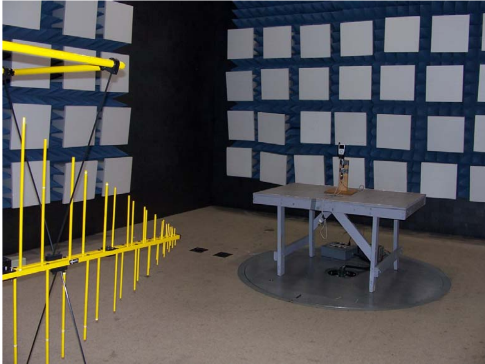
Figure 1- Photo of Part 15.209 testing set up (Front)
