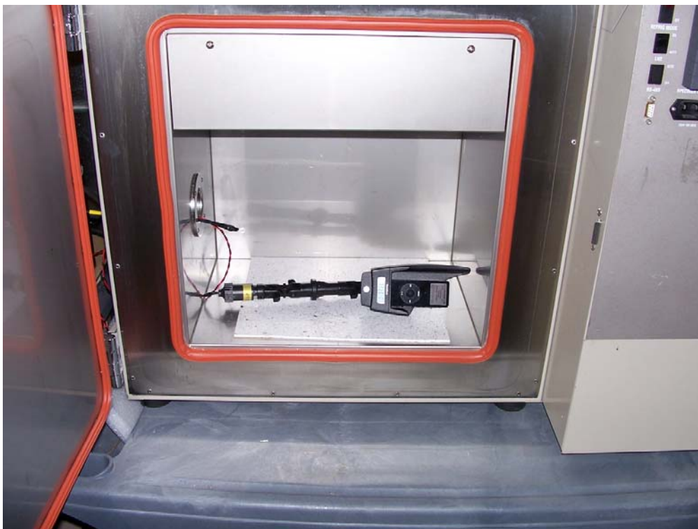
Figure 14 – Shows the use of the ipod nano for Frequency stability over temperature variations.
