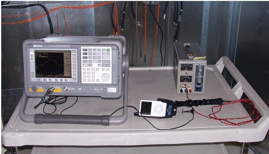
Figure 9- Setup for Bandwidth testing and Frequency Stability over Voltage Variations.
