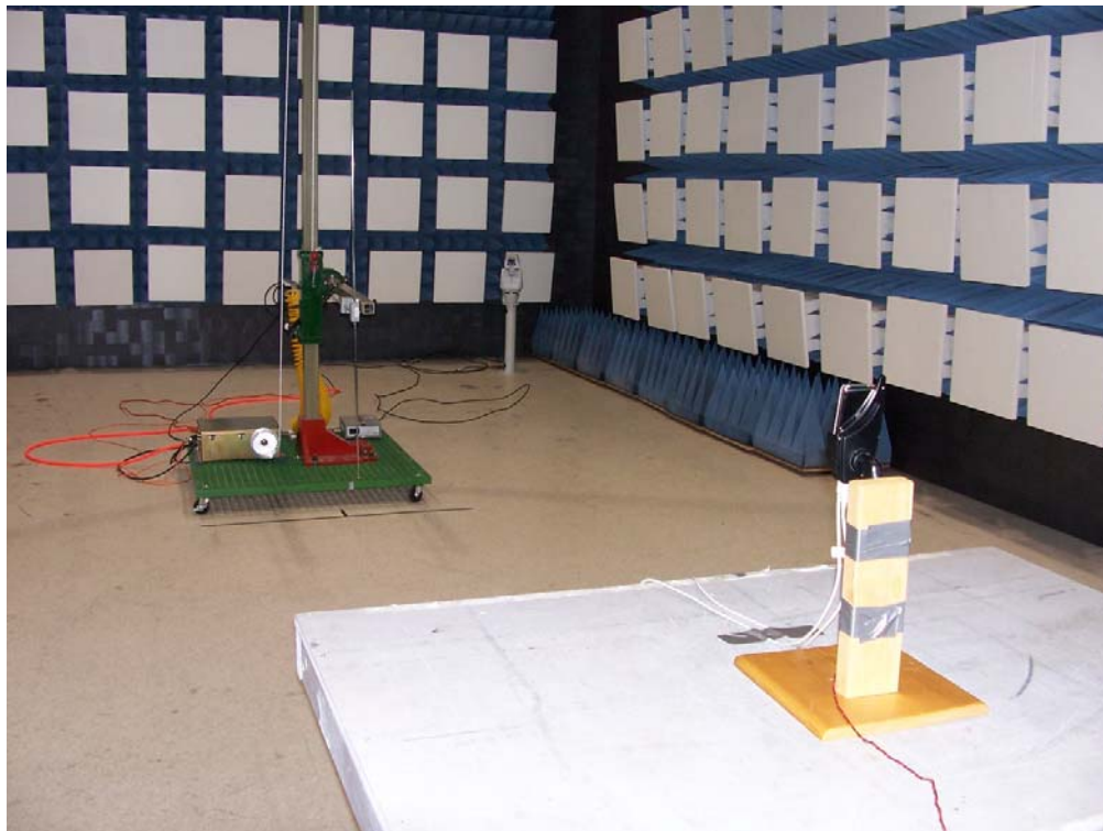
Figure 4 - Photo of Part 15.209 testing set up (Back)
