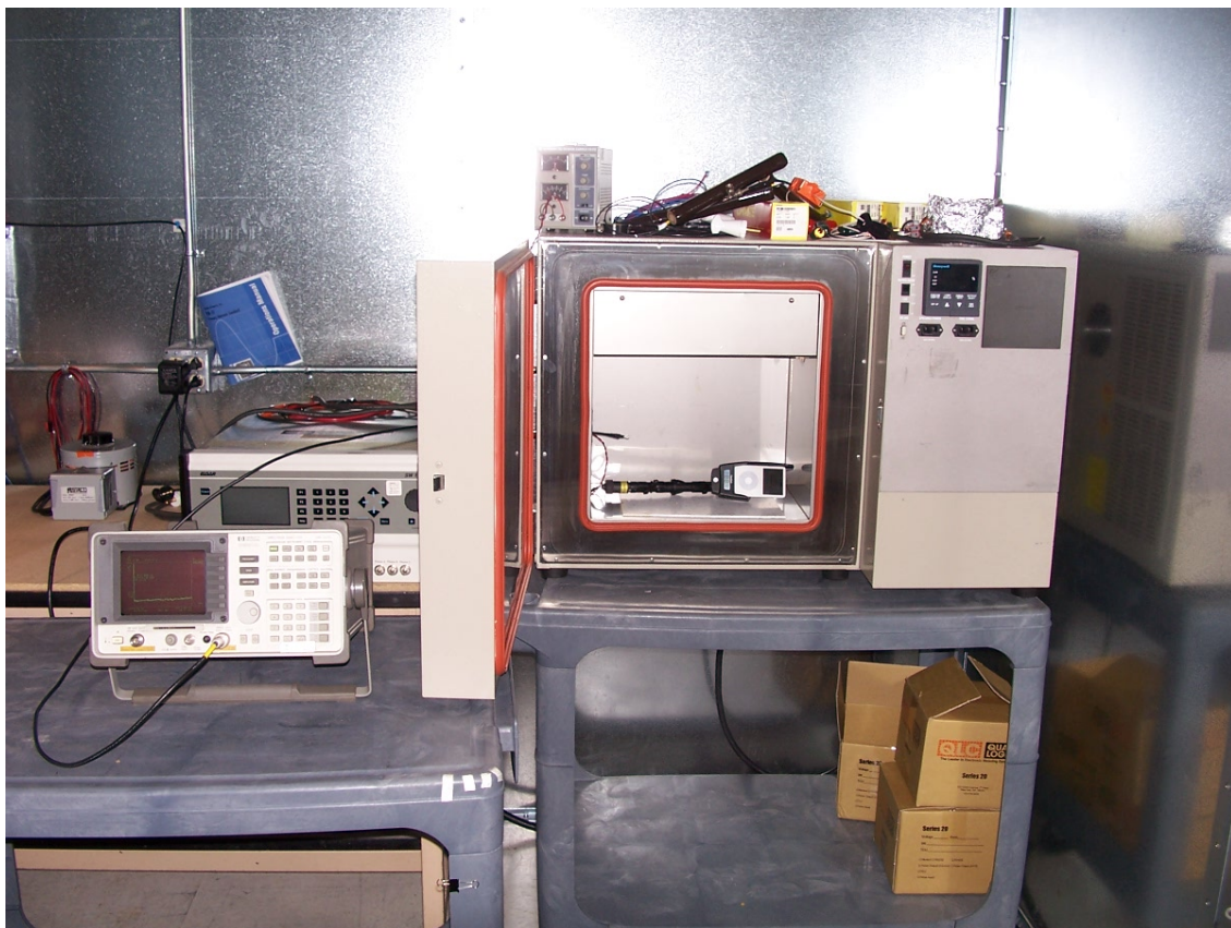
Figure 10 – Setup for Frequency Stability over Temperature Variation Measurements.
