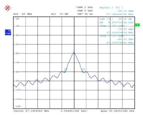
Down 20dB Bandwidth: 4.4KHz (27.1432MHz to 27.1476MHz)
